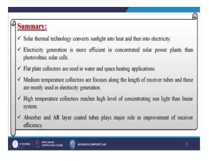
Now, we have come to the last part of this particular lecture where basically in summary we can say that solar thermal technology converts the sunlight into heat and then into electricity. The electricity generation is more efficient in concentrated solar power plants than photovoltaic solar cells. Flat plate collectors are used in water and space heating applications.
