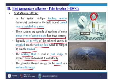
Next is called the third one which is nothing, but the high temperature collectors or it is known as also point focusing which is basically more than 400 degree centigrade. So, that is also divided into several parts, one is called the central tower collector.
