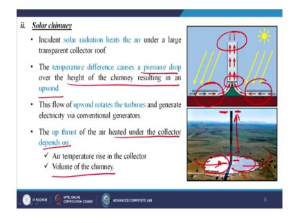
Next come to the solar chimney. So, incident solar radiation hits the air under a large transparent collector roof. The temperature difference causes a pressure drop over the height of the chimney resulting in an upwind.
