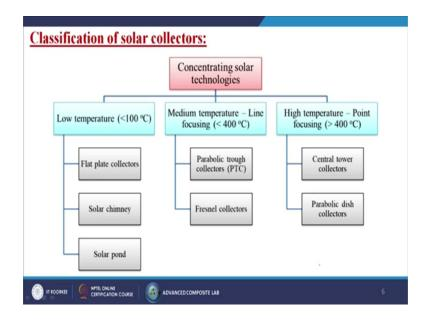
So, basically what are the classifications of the solar collectors? First concentration solar technologies it has been divided into 3 parts, first is called the low temperature which is nothing, but below 100 degree centigrade, medium temperature or may be the line focusing which is below 400 degree centigrade, another one is known as the high temperature or maybe the point focusing which is more than 400 degree centigrade.
