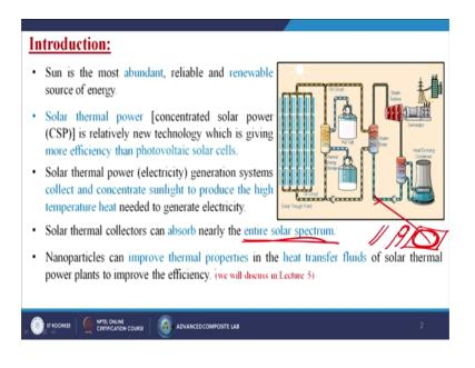
So, basically the solar thermal power, concentrated solar power basically, because why I am talking this one is the consented because I will come into the subsequent slides. Basically, in this particular case we are using some kind of mirror or maybe the reflecting glasses so that the whole energy solar energy basically we are concentrating in a particular point and then we are focusing that particular solar energy into the systems. So, here the consumption of the solar energy is more.
