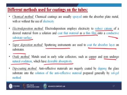
So, now there are different methods used for coatings on the tubes. What are those? First one is known as the chemical method. So, in the chemical coatings are usually sprayed onto the absorber plate metal with or without the use of electricity. So, simple you are doing a coating on to the material or may be the substrate.
