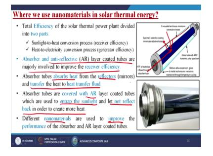
Now, one basic question, that why or maybe where basically we are using the nano materials for solar thermal energy generations. So, total efficiency of the solar thermal power plant divided into two parts, one is called the sunlight to heat conversion process or maybe the receiver efficiency and second one is known as the heat to electricity conversion process or maybe sometimes it is known as the generator efficiency.
