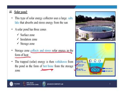
Next let us discuss about the solar pond. This type of solar energy collected uses a large salty lake that absorbs and stores energy from the sun. So, basically seawater which is nothing but the brine solutions also that is the mixing of the water with the sodium chloride. So, basically, we are using that technology over here.
