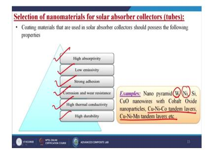
Now, what will be the basic for selection of nanomaterials for solar absorber collectors or may be the tubes? How? Which kind of materials we can choose? What are the criterias?
