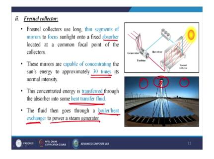
Next is called the Fresnel collector. So, Fresnel collectors use long thin segments of mirrors to focus sunlight onto a fixed absorber located at a common focal point of the collectors itself.
