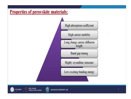
So, if we talk about the properties of perovskite materials. So, basically these materials is having high absorption coefficient, high carrier mobility, long charge carrier diffusion length, band gap tuning, highly crystalline structure and the low exciting binding energy. So, these all properties are very very useful for making any kind of solar cells.
