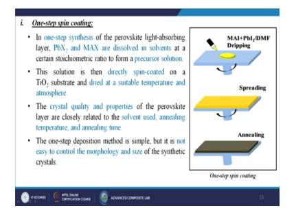
So, basically if you talk about the one step spin coating, in one step synthesis of the perovskite light absorbing layer PbX 2 and MAX are dissolved in solvents at a certain stoichiometric ratio to form a precursor solution.
