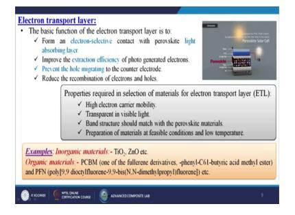
So, what is electron transport layer? So, the basic function of the electron transport layer is to form an electron selective contact with perovskite light absorbing layer; improve the extraction efficiency of auto generated electrons; prevent the whole migrating to the counter electrode; reduce the recombination of electrons and the holes.
