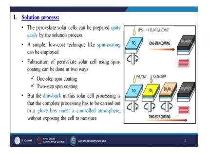
So, the perovskite solar cells can be prepared quite easily by the solution process a simple low cost technique like spin coating generally we are doing this particular process by using the spin coater. So, a simple low cost techniques like spin coating can be employed, fabrication of perovskite solar cell using spin coating can be done in two ways as I told already one is called the one step spin coating, another one is called that two step spin coating.
