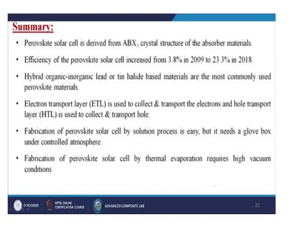
So, we have reached to the last slide of this particular lecture. So, in summary I can say that perovskite solar cells is derived from the ABX 3 crystal structure of the observer materials right. Efficiency of the perovskite solar cells increased from 3.8 percent in 2009 to 23.3 percent in the year of 2018 and till today it is 23.7 percent.
