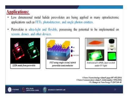
Low dimensional metal halide perovskites are being applied in many optoelectronic applications such as FETs, photo detectors and the single photon emitters. Perovskite is ultra light and flexible processing the potential to be implemented on screens drones and other devices. So, any kind of shapes simply you can stick that particular materials. So, it will be the flexible one.
