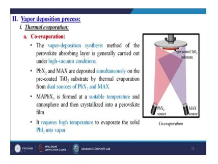
Next this vapor deposition process. So, basically from the name itself you can understand that it is a one kind of thermal evaporation process. So, basically that is also divided into several parts the first one is known as the co evaporation process. So, the vapor deposition synthesis method of the perovskite absorbing layer is generally carried out under high vacuum conditions. So, high vacuum means there is a less chance of the perovskite materials to degrade.
