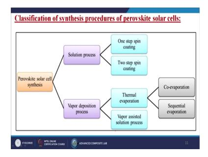
Now if we talk about the classification of synthesis procedures of the perovskite solar cells. So, basically the synthesis process is divided into two parts; one is called the
