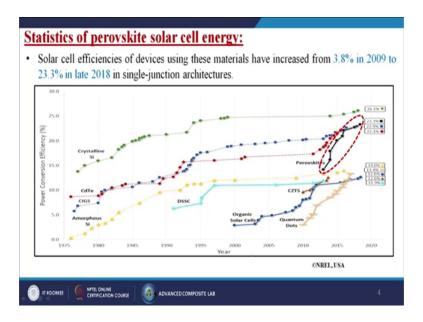
So, now if we talk about the statistics of the perovskite solar cell energy, so, solar cell efficiencies of devices using this materials have increase from 3.8 percent in 2009 to 23.3 percent in late 2018 in single junction architectures. So, now, you can see 1975 to 1980 we are using the amorphous silicon CIGSs CdTe crystalline silicon which already I have discussed in lecture 2. So, now, when we are going towards the 21st century so, you can
