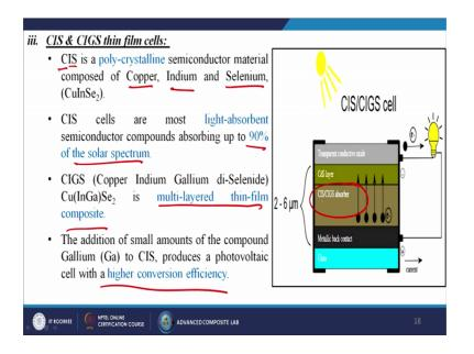
Next we are having that CIS and CIGS thin film solar cells. So, CIS is a polycrystalline semiconductor material composed of C stands for Copper, I stands for Indium and S stands for Selenium. So, basically it is the copper indium di selenide. So, CIS cells are most light absorbing semiconductor compounds, absorbing up to 90 percent of the solar spectrum. CIGS: Copper Indium Gallium di-Selenide is multilayer thin film composite materials.
