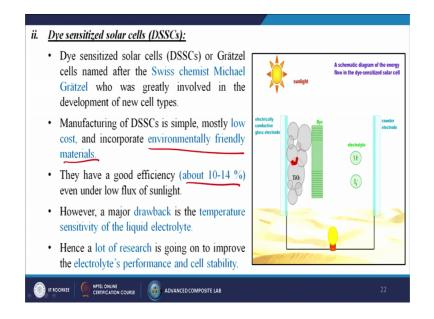
Next we are having the dye sensitized solar cells; till today maximum cases we are using this means maximum applications basically we are using the dye sensitized solar cells. So, basically the dye sensitized solar cells in short DSSC or maybe the Gratzel cells named after the Swiss chemist Michael Gratzel, who was greatly involved in the development of new cell types.
