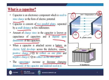
Now, before going to discuss about the super capacitors, just let us know what is capacitors. Capacitor is an electronic component which is used to store charge in the form of electric potential. Capacitor is consists of two parallel plates separated by a small distance in few millimeters. Amount of charge store in the capacitor is known as capacitance of capacitors and is depend upon dimensions of the capacitors itself.
