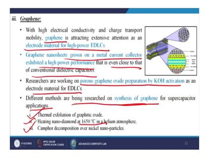
Next, we are using the grapheme, so basically with high electrical conductivity and charge transport mobility, graphene is attracting extensive attention and as an electrode material for high power EDLC. Graphene nanosheets grown on a metal current collector exhibited a high power performance that is even close to that of conventional electric capacitors.
