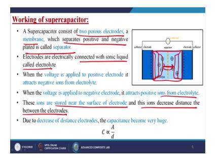
Now, working of the super capacitor, a super capacitor consists of two porous electrodes a membrane, which separates positive and negative plated is called the separator. Electrodes are electrically connected with ionic liquid called the electrolyte. So, this area is totally filled by this electrolyte, so this area basically. When the voltage is applied to positive electrode, it attracts negative ions from the electrolyte, so negative ions are coming over here.
