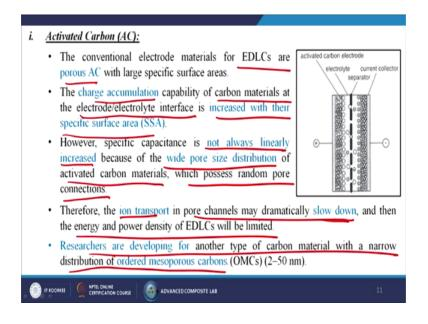
What kind of materials basically, we can use? Maximum cases we are using the activated carbon. The conventional electrode materials for EDLCs are porous activated carbon with large specific areas. The charge accumulation capability of carbon materials at the electrode electrolyte interface is increased with the specific surface area.
