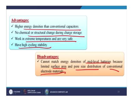
What are the advantages? High energy densities than conventional capacitors, no chemical or structural change during charge storage, work in extreme temperatures and are very safe, have high cycling stability. Of course, there are certain disadvantages cannot match energy densities of mid level batteries because limited surface area and pore size distribution of conventional electrode materials.
