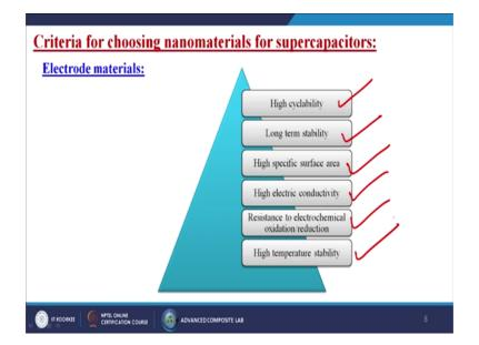
Now, what are the criteria? Not maybe the what are the parameter for choosing the nano materials for super capacitor. If we talk about the electrometer electrode materials point of view we need the high cyclability, long term stability, high specific surface area, high electric conductivity, resistance to electric electrochemical oxidation or maybe the reduction and the high temperature stability.
