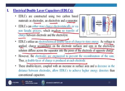
Now, let us discuss on Electrical Double Layer Capacitors or it may be the in short it is called the EDLC. EDLC are constructed using two carbon based materials as electrodes, an electrolyte and the separator. So, simple both are carbon based, so that is why it is c 1 and c 2. One will be the positive one, another will be the negative one; in between that we are using the separator and we are using the electrolyte.
