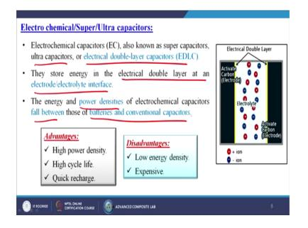
Next one is the electrochemical or maybe the super or may be the ultra capacitors; electrochemical capacitors are known as super capacitors, ultra capacitors or electrical double layer capacitors in short basically we are calling it as a EDLC. So, in this particular case you can see that we are using two electrode over there; both are made by the activated carbon electrode and inside that we are putting the electrolytes.
