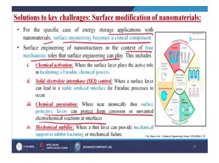
So, for the specification of energy storage applications with nano materials; surface engineering becomes a critical component. Surface engineering of nano structures in the context of four mechanistic roles that surface engineering can play. This includes the number one; chemical activation where the surface layer plays the active role in facilitating a Faradaic chemical process.
