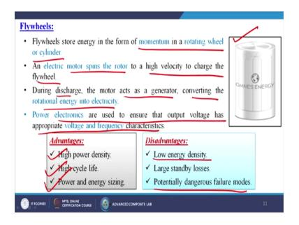
Next come to the flywheels; flywheels store energy in the form of momentum in a rotating wheel or cylinder; which you can see from this particular image. And electric motors spins the motor to a high velocity to charge the flywheel; during discharge the motor acts as a generator converting the rotational energy into electricity. Power electronics are used to ensure that output voltage has appropriate voltage and frequency characteristics.
