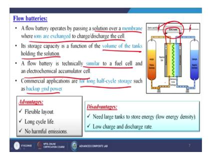
So, a flow battery operates by passing a solution over a membrane where the ions are exchanged to charge discharge the cell; so, basically this green in colour is called the membrane. So, in this particular case we are having that positive electrode, we are having that negative electrode. So, in this particular case what is happening? It is aligned to go the ions from one site to another site, but it is abstracting to move the electrons through that particular membrane.
