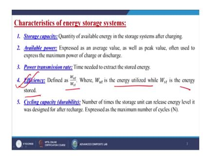
Now; what is the characteristics of energy storage systems? So, first one is called the storage capacity; storage capacity is nothing, but the quantity of available energy in the storage systems after charging; that means, it is like a tank. So, just I am pouring the water; so at the end of the day; how much quantity or may be volume of water I am storing inside that particular tank?
