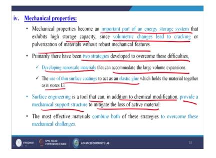
Now, the last one is the mechanical properties; mechanical properties become an important part of an energy storage system that exhibits high storage capacity, since volumetric changes lead to cracking or pulverization of material without robust mechanical features.
