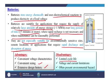
Now, we are going to discuss about the batteries. So, battery store energy chemically and use electrochemical reactions to produce the electricity at a fixed voltage. In class may be 10 or may be 12; we have already gone through the working principle of the batteries.
