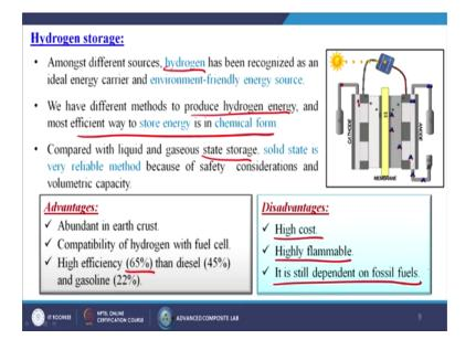
Next one is called the hydrogen storage; amongst different sources hydrogen has been recognized as an ideal energy carrier and environment friendly energy source. In our future slides, we are going to deliver one lecture totally based on the hydrogen storage systems.
