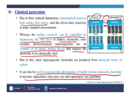
The next one is called the chemical passivations; due to their reduced dimensions nano materials possesses high surface free energy and this drives their reactivity in many standard environments. So, in this particular case what we are doing? Simple we are doing the coating of the graphene layer there. So, we are having pristine P Si materials, highly doped silicon basically we are using and in between that the electrolytes are there.
