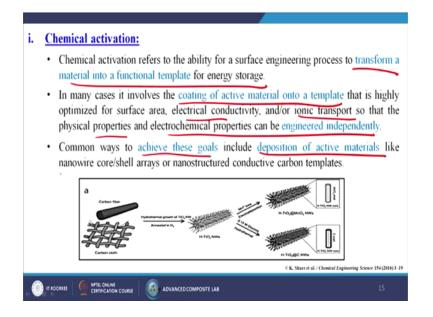
Now, what is chemical activations? So, basically chemical activations refers to the ability of a surface engineering process to transform a material into a functional template for energy storage.
