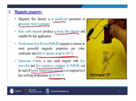
Now, it depends upon the magnetic property. Magnetic flux density is a significant parameter in designing micro generator. Rare earth magnets produces strong flux density and suitable for these particular applications. Neodymium iron boron magnets is known as most powerful magnetic properties per cubic centimeter and able to operate at up to 140 degree centigrade.
