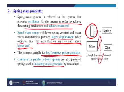
Next one is called the spring-mass property. So, basically the spring-mass system is referred as a system that provides the oscillations for the magnet in order to achieve flux cutting mechanism and induce certain emf. Spiral shape spring with lower spring constant and lower stress concentration produce larger displacement when oscillate, thus maximize flux cutting rate and induce the higher emf.
