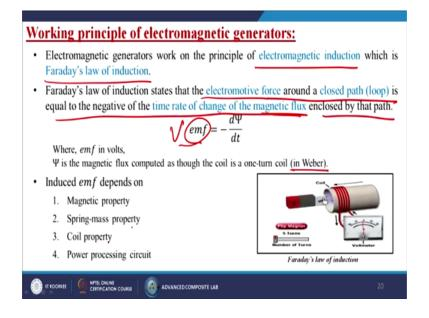
Now, what is the working principle of electromagnetic generators? Basically the electromagnetic generators work on the principle of electromagnetic induction, which is Faraday's law of induction. Faraday's law of induction states that the electromotive force around a closed path or loop is equal to the negative to the time rate of change of the magnetic flux enclosed by that particular path.
