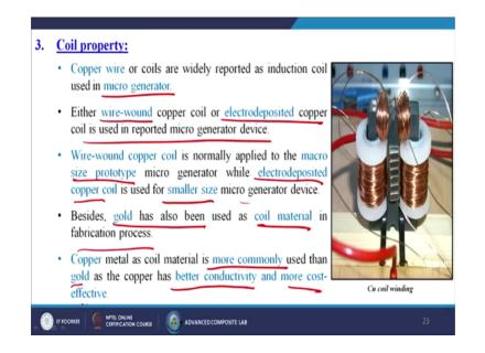
Next one is called the coil property. So, basically the copper wire or coils are widely reported as induction coil used in micro generator. Either wire-wound copper coil or electrodeposited copper coil is used to reported micro generator device. Sometimes we are doing certain kind of coating on to the copper coil also. Wire-wound copper coil is normally applied to the macro size prototype, micro generator while electro deposited copper coil is used for smaller size micro generator device.
