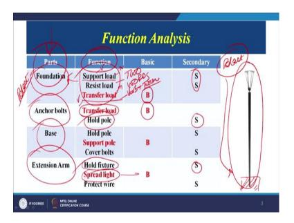
Now, let us take the functional analysis here this is a lamp post you can see. So, we can have a foundation here for this lamp post. So, we have seen first we have to blast the product which is a lamp post into the individual components. So, here you can see one of the important parts or components of this product is the foundation, then there are anchor bolts, then there is a base, then there is an extension arm, then there is housing or a fixture and then there is a light bulb.
