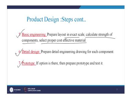
Then, the basic engineering will be done on that, we will prepare, the layout on a exact scale, calculate the strength of the component, select the proper cost effective material. So, material selection component design, part design, part assembly all these decisions will be taken at the basic engineering level.
