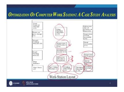
So, let us quickly now see. This is just the information collection, workstation layout how this is being manufactured; the authors have given a very clear idea about what are the machines. So, there is a edge binding machine available, then inspection of the product is done at this location, packaging of goods, storage, and this is a place from where the materials will be dispatched.
