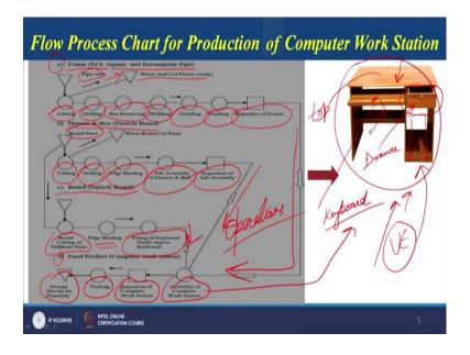
Then this is a flow process chart, this is a computer table how it will look like, we can see if this is a drawer here, this is the top of the table, this is a place to keep the keyboard. So, first thing is we need to have, a complete understanding of the computer table. This is a place where CPU will be placed then, this is another shelf to keep certain important thing.
