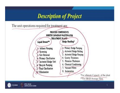
Now, this is a description of the project, the unit operations required for the treatment are, so what are the requirements we can see here, there is a liquid stream, and there is a sludge handling stream. So, this is star for ultimate capacity of the plant and double star is for the average flow that is required.
