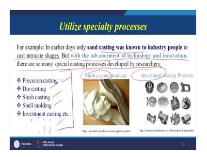
For example, in earlier days only sand casting was known to the industry people to cast the intricate shapes. But with, the advancement of technology and innovation there are so many special casting processes developed by researchers. Like precision casting, die casting, slush casting, shell molding casting, investment casting, so many casting process and even this list is endless there can be other casting processes also.
