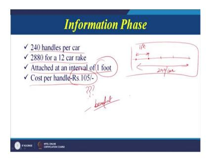
So, there are 240 handles per car, 2880 for a 12 car rake, then attached at an interval of 1 foot, cost per handle is rupees is 105. So, which means that suppose this is a rod, this is one handle; this is another handle, the distance between the handles is 1 feet and their number is also listed. So, this total number is 240 per car, and the total number is also
