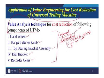
So, now let us take this example of a universal testing machine which has been published. So, the source is given at the end of the presentation. So, the application of value engineering for cost reduction of universal testing machine. So, value analysis technique for cost reduction of following components of UTM.
