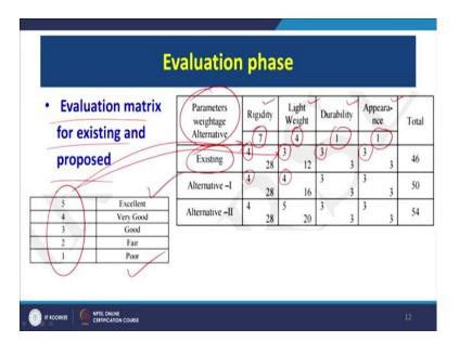
Now, here we can see the evaluation matrix for the existing and the proposed; this is the ranking 5, 4, 3, 2, 1; 5 is excellent, 1 is poor. So, we can see here, parameters weightage so, rigidity, lightweight, durability and appearance. So, this is the ranking 7, 4, 1 and 1 which we have found out in the previous slide. If you can go back to the previous slide and 7, 4, 1, so, existing we are giving the ranking rigidity is 4, lightweight is 3 ranking.
