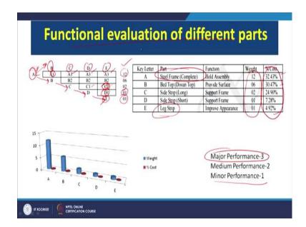
So, we can see that once we do this functional evaluation of the different parts, we can see hold the assembly the weight is also given, percentage cost contribution is also given. So, what we do? We do in context of B, C, D and E. So, if you go back, you can see. We have named these parts as A, B, C, D and E. So, in our analysis part we have tried to relate. So, three basically wherever we have written it means that A and B are strongly dependent; so major performance.
