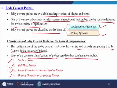
Second Eddy Current Probes: Eddy current probes are available in a large variety of shapes and size. One of the major advantages of eddy current inspection is that probes can be custom designed for a wide variety of applications. So depending upon the sample size, depending upon the material size, there are different types of probes are available. Eddy Current Probes are classified on the basis of configurations of the test coils and the mode of operation.
