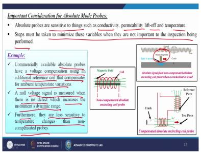
Important considerations for Absolute mode probes: Absolute probes are sensitive to things such as conductivity, permeability, liftoff and the temperature. Steps must be taken to
