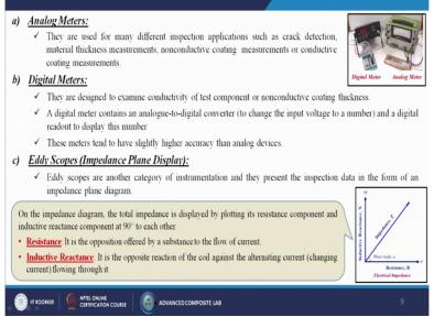
What is Analog Meter? They are used for many different inspection applications such as crack detection, material thickness measurements, non conductive coating measurements or maybe the conductive coating measurements. Next come to the digital meters, so here you can see, that digital meters, the value will come digitally and analog meter maybe some graph
