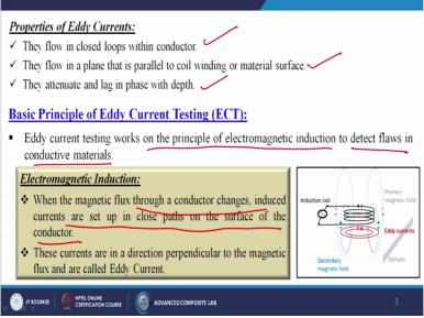
Properties of the Eddy Currents: They flow in closed loops with conductor. They flow in a plane that is parallel to coil winding or maybe the material surface. They attenuate and lag in phase with depth. Now what are the basic principles of the Eddy current testing? Eddy current testing works on the principle of electromagnetic induction to detect flaws in conductive materials.
