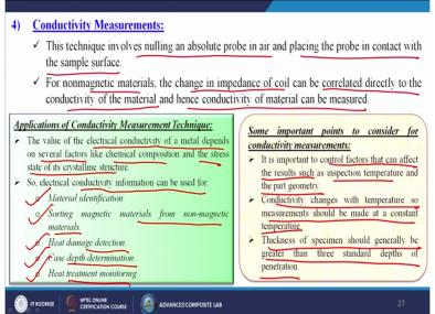
Next Conductivity Measurements, these techniques involves nulling an absolute probe in air and placing the probe in contact with the sample surface. For non-magnetic materials, the change in impedance of coil can be correlated directly to the conductivity of the material and hence conductivity of material can be measured, applications of conductivity measurement techniques.
