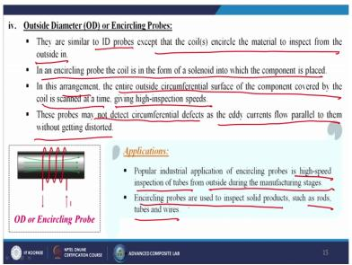
Next Outside Diameter or may be the Encircling Probes. They are similar to ID probes except that the coils encircle the material to inspect from the outside in. In an encircling probe the some oil is in the form of a solenoid into which component is placed. In this arrangement the entire outside circumferential surface of the component covered by the coil is scanned at a time giving high inspection speeds. So that means one is internally we are putting and one is externally we are putting.
