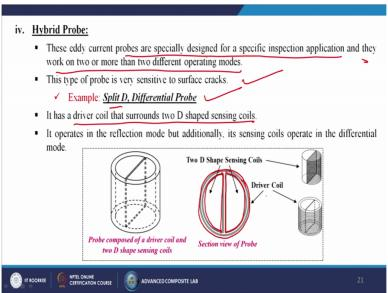
Next is called the Hybrid probe. These eddy current probes are specially designed for a specific inspection application and they work on two or more than two different operating modes. This type of probe is very sensitive to surface cracks. Example: Split D, Differential probe. It has a driver coil that surrounds two D shaped sensing coils here. So this is one D and this is another D and this is surrounded by the driver coil.
