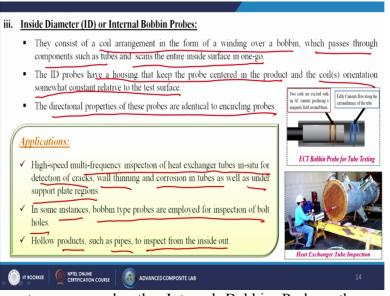
Third Inside Diameter or may be the Internal Bobbin Probes, they consist of a coil arrangement in the form of a winding over a bobbin, which passes through components such as tubes and scans the entire inside surface in one go. The ID probes have a housing that keeps the probe centered in the product and the coils orientation somewhat constant relative to the test surface.
