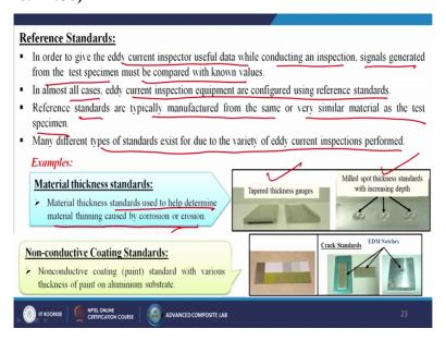
Now come to the Reference Standards. What is reference standards? In order to give the eddy current inspector useful data while conducting an inspection, signals generated from the test specimens must be compared with the known values. Yes of course, known values means, some standard values. In almost all cases eddy current inspection equipments are configured using reference standards. Reference standards are typically manufactured from the same or very similar material as the test specimen.
