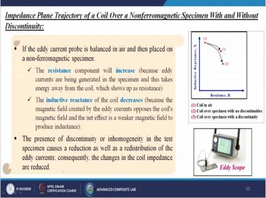
Now Impedance Plane Trajectory of a Coil over a Non ferromagnetic Specimen with and without the discontinuity. If the eddy current probe is balanced in air and then placed on a non ferromagnetic specimen, the resistance component will increase, because eddy currents are being generated in the specimen, and this takes energy away from the coil, which shows up as resistance.
