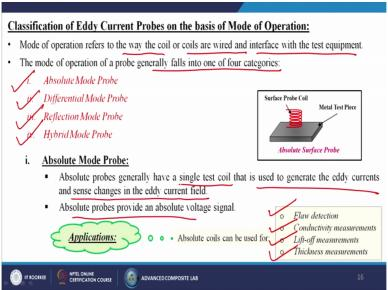
Classification of Eddy current probes on the basis of mode of operations: Mode of operations refers to the way the coil or coils are wired and interface with the test equipment. The mode of operation of a probe generally falls into one of four categories. What are those? Absolute mode probe, Differential mode probe, Reflection mode probe and the Hybrid mode probe. So now, first we are going to discuss about the, Absolute mode probe.
