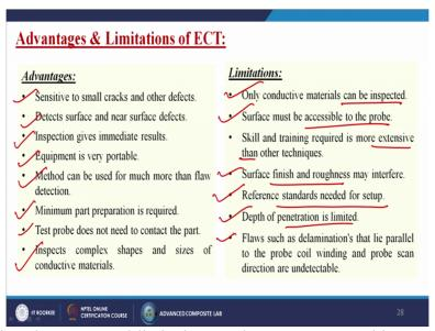
Now what are the advantages and limitations? Advantages are sensitive to small cracks and other defects. Detects surface and near surface defects. Can be easily measured, inspection gives immediate results. Equipment is very portable. Handy method can be used for, much more than flaw detection. A minimum part preparation is required. Test probe does not need to contact the part inspects complex shapes and sizes of conductive materials.
