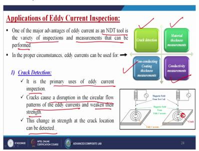
Now applications of the Eddy current inspection: One of the major advantages of eddy current as an NDT tool is to variety of inspections and measurements that can be performed. In the proper circumstances, eddy currents can be used for crack detection, material thickness measurements, conductivity measurements, non conducting coating thickness measurements. What is crack detection? It is the primary uses of eddy current inspections. Cracks cause a
