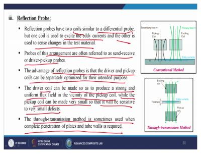
Next come to the third one that is called the Reflection Probe. Reflection probe have two coils similar to a differential probe but one coil is used to excite the eddy currents and the other is used to sense changes in the test material. Here not both the probes are, testing the
