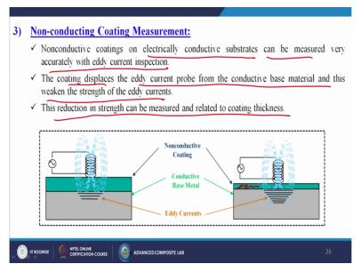
Non-conducting Coating Measurement, Non conductive coatings on electrically conductive substrates can be measured very accurately with eddy current inspections. The coating displaces the eddy current probe from the conductive base material and this weakens the strength of the eddy currents. This reduction in strength can be measured and related to the coating thickness. So these green in color is the coating thickness, this is the conductive base metals. So this will weaken the signal.
