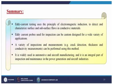
Now we have come to the last slide of this particular lecture. So as a summary, we can say, that eddy current testing, use the principle of electromagnetic induction which has been developed by Faraday to detect and characterize surface and subsurface flaws, in the conductive material. Eddy current probes used for inspections can be custom designed for a wide variety of application. It is totally depends upon your shape and size you can customize your own probe.
