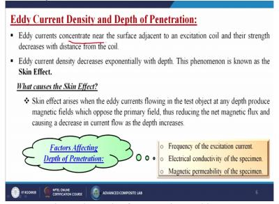
Next is Eddy Current Density and Depth of Penetration: Eddy currents concentrate near the surface adjacent to an excitation coil and their strength decreases with distance from the coil. So that means, a thin sample can be easily detected rather than the thick sample. Eddy current density decrease exponentially with the depth. This phenomenon is known as the Skin Effect.
