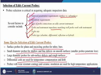
Now selection of Eddy current probes: Probe selection is critical in acquiring adequate inspection data. Several factors to consider include, material penetration requirements, surface versus subsurface, sensitivity requirements, types of probe connections on eddy current instrument, probe and instrument impedance matching will probe work with instrument, next is the probe size, and last one is the probe type whether it is absolute, differential, reflection or maybe the hybrid.
