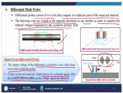
Next come to the Differential mode probe: Differential probes consist of two coils that compare two adjacent parts of the inspected materials. The detecting coils are wound in the opposite directions to one another in order to equalize the induced voltage originated by the excitation primary field. Now differential double functioning in circle coil is looking like this.
