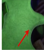
Gear with Service Induced Crack
