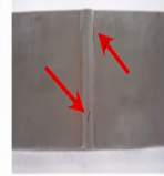
Throat and Toe Cracks in Partially Ground Weld
