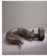
Crane Hook with Service Induced Crack
