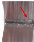
Lack of Fusion in SMAW Weld
