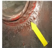
Crack in Seal Weld of Boiler Tube to Steam Drum
