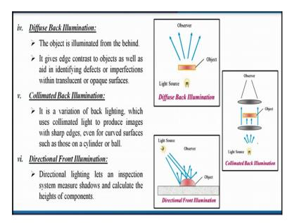
Next one is called the diffusive, diffuse back illumination. So, the object is illuminated from the behind. It gives edge contrast to objects as well as aid in identifying defects or imperfections within translucent or opaque surfaces. So, in this case, the light source is behind the object and through that the light is coming to the observer eyes.
