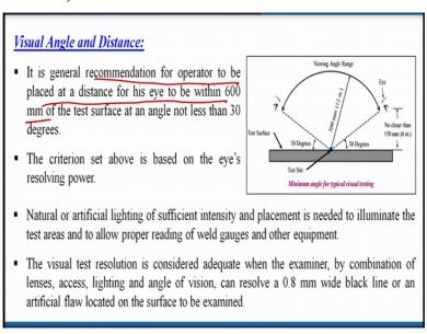
Next how we can do this particular experiment. So generally, it is general recommendation for operator to be placed at a distance for his eye to be within 600 millimeters of the test surface at an angle not less than 30 degrees. Say suppose this is your total sample right, so in this particular sample you can see up to the maximum 300 millimeters or maybe the 12 inches so, up to 12-inch distance you can see that material clearly and the angle should be within this range.
