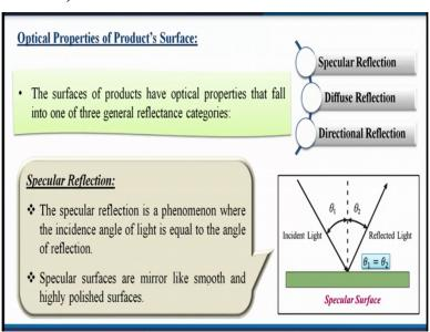
Optical properties of products surface. So generally, the surface of products have optical properties that fall into one of three general reflectance categories. What are those? First one is called the Specular Reflection, second one is called the diffuse reflection and third one is called the directional reflection. What is specular reflection?
