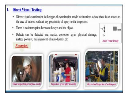
So, when you talk about the direct visual testing. Direct visual examination is the type of examination made in situations where there is an access to the area of interest without any possibility of injury to the inspector. That means we can directly see that particular zone. There is no interruption between the eye and the object. Defects can be detected are cracks, corrosion layer, physical damage, surface porosity, misalignment of mated parts etc.
