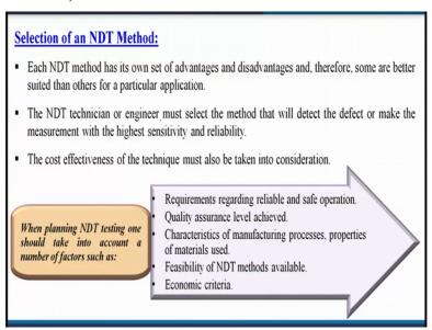
Now, how to select. That which method or may be the which technique is best for this particular testing. Because they have, I have told already there are n number of testing. But it is not possible that every time to do all testing for a particular material. So, depends upon the applications, it depends upon the material properties, it depends upon the which kind of materials to or you are going to use or may be where you are going to use.
