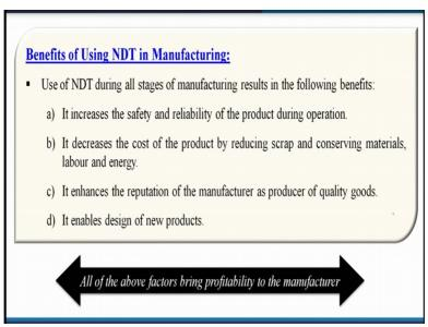
Now what are the benefit of using NDT in manufacturing techniques. So first, it increases the safety and reliability of the product during operation. It decreases the cost of the product by reducing scrap and conserving materials, labor and energy. It enhances the reputation of the manufacturer as producer of quality goods. It enables design of new products. But one thing I can tell you that NDT testing does not means that material will never fail in future.
