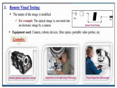
Next, remote visual sensing. The nature of the image is modified. Suppose in our surface a very tiny crack or maybe the small crack is there, but we cannot see it eye, by our naked eyes so that time we are using some kind of techniques which is zooming that particular zone and by zooming or getting the zooming figure we are getting some kind of information about that particular materials.
