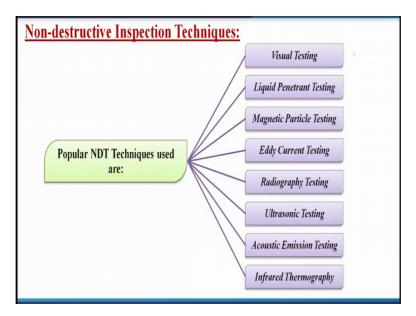
Now, what are the techniques? So, there are so many techniques are available but most popular techniques are like that visual testing, liquid penetrant testing, magnetic particle testing, eddy current testing, radiography testing, ultrasonic testing, acoustic emission testing and infrared thermography.
