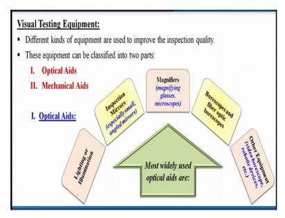
Now, what are the instrument? Different kinds of equipment are used to improve the inspection quality. These equipment can be classified into two parts; one is called the Optical aids and the second one is called the mechanical aids. So, what is optical aids? So generally, there are several types of optical aids are available.
