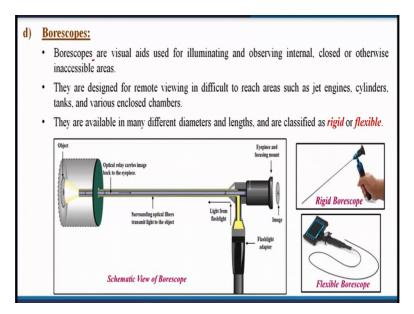
Next is called the borescopes. So, borescopes are visual aids used for illuminating and observing internal, closed and otherwise inaccessible areas. They are designed for remote viewing in difficult to reach areas such as jet engines, cylinders, tanks, and various enclosed chambers. They are available in many different diameters and lengths, and are classified as rigid or maybe the flexible. So, this is the schematic view of the borescope.
