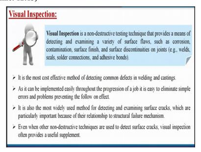
So generally, the visual inspection is a nondestructive testing technique that provides a means of detecting and examining a variety of surface flaws, such as corrosion, contamination,
