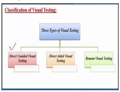
Now there are three distinct classification of the visual testing. So, number 1 is called the direct unaided visual testing, second one direct aided visual testing and the third one is the remote visual testing.
