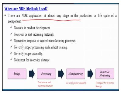
When we are using the NDE method? There are NDE application at almost any stage in the production or life cycle of a component. As I told already, to assist a product development, to screen or sort incoming materials, to monitor, improve or control manufacturing processes. To verify proper processing such as heat treating, to verify proper assembly to inspect for in service damage.
