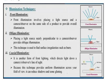
Next illumination techniques. So, there are different types of illumination techniques available. First one is called the front illuminations. So, from front illuminations involves placing a light source and a camera observer on the same side of a product to provide the overall illuminations. So, that is called the front illuminations. So, here I am having that object, and the light is coming and the observer eyes over here so that is known as the front illuminations.
