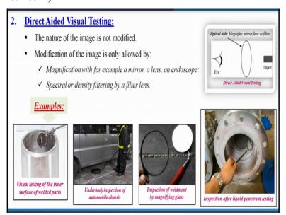
Next, we are coming to direct aided visual testing. So, from the name itself you can understand that aided part has been added; that means with the help of something. So, the nature of the image is not modified. Modifications of the image is only allowed by
