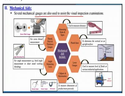
Next second one is the mechanical aids. Several mechanical gauges are also used to assist the visual inspection examinations. So, those are some kind of screw pitch gauge, some kind of angle measuring tool, outside caliper, Vernier caliper, micrometer, level indicator.
