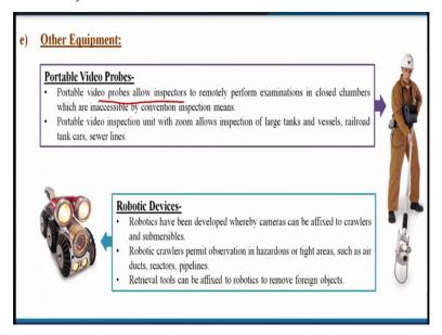
Other equipment like portable video probes. Portable video probes allow inspectors to remotely perform examinations in closed chambers which are inaccessible by convention
