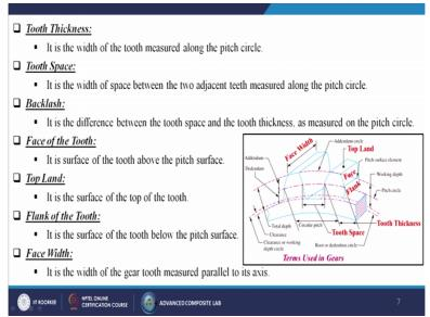
Now come to the tooth thickness it is the width of the tooth measured along the pitch circle. So, now when we are seeing this one is known as the tooth thickness over there now tooth space it is the width of space between the two adjacent teeth measured along the pitch circle. So, now we are having that tooth space is this one and two thickness is this one. This is the thickness of the tooth and this is the gap in between the two gears that is known as the tooth space.
