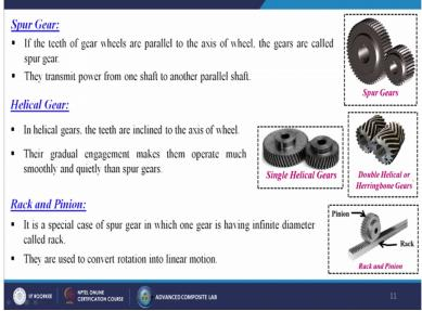
So, now what is spur gear if the teeth of the gear wheels are parallel to the axis of the wheel the gears are called spur gear they transmit power from one shaft to another parallel shaft you see they are mating front to front. Next come to the helical gear in helical gears that teethes are inclined to the axis of wheel their gradual engagement makes them operate much smoothly and quietly than the spur gears.
