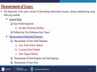
Now come to the measurement of gears then how we can measure that about the gear teeth and all the details. So, the inspection of the gears consists of determining the dimensional accuracy during manufacturing using the following methods. First one is the general tests what are those gear profile impact inspections like involute measuring machine and the second one is the rolling gear test that is known as the Parkinson gear tester.
