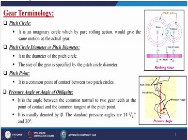
So, now come to the gear terminology let us know in depth about that gear. So, what is pitch circle it is an imaginary circle which by pure rolling actions would give the same motions as the actual gear. So, now I am having the driver, driver means it is an engine so it is rotating and whichever it is rotating that is known as the follower. So, this is the pitch circle over there in these particular cases so where it is mating at the center.
