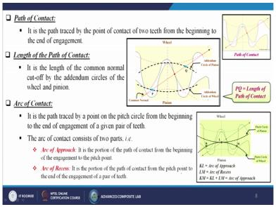
Then path of contact it is the path traced by the point of contact of two lengths from the beginning to the end of the engagement so that is the path of contact. Length of the path of contact it is the length of the common normal cut off by the addendum circles of the wheel and pinion. Arc of contact it is the path traced by a point on the pitch circle from the beginning to the end of the engagement of a given pair of teeth.
