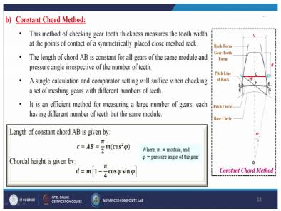
Next is called the constant quad method this method of checking gear to thickness measures the tooth width at the points of contact of a symmetrically placed close missed rack. The length of chord AB is constant for all gears of the same module and pressure angle is irrespective of the number of teeth. A single Galatians and comparator setting will suffice when checking a set of machine gears with different numbers of teeth.
