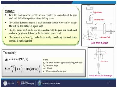
Working principles so in this particular case first the blade position is set to a value equal to the addendum of the gear tooth and locked into position with a locking screw the caliper is set on the gear in such a manner that the blade surface snugly fits with the top surface of the gear teeth. So, now you can see that it is rigidly tighting your gear teeth. The two anvils are brought into the close contact with the gear and the chordal thickness is noted down on the horizontal vernier scale.
