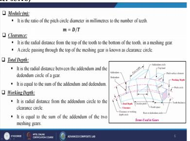
Next come to the module m it is the ratio of pitch circle diameter in millimeters to the number of teeth so m=D/T then come to the clearance because if we do not put the clearance so high friction will be generated and there is a chance that gear teeth can break so that is why you are giving certain kind of clearance or maybe the tolerance value over there. So, it is the radial distance from the top of the tooth to the bottom of the tooth in a meshing gear.
