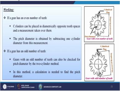
Now working principles if a gear has an even number of teeth cylinders can be placed in diametrically opposite to spaces and measurement taken over them so easy so one is here and another one is here so this is the measured readings over there this is the cylindrical plug and this is the pitch diameter over there. So, the pitch diameter is obtained by subtracting one cylinder diameter from this particular measurement so easily we can measure.
