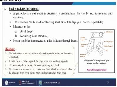
Next one is the pitch checking instrument so pitch checking instrument is essentially a dividing head that can be used to measure pitch variations. The instrument can be used for
