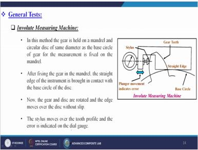
So, first let us discuss about the general tests so when you are talking about the involute measuring machines in this method the gear is held on a mandrel and the circular disc of same diameter as the base circle of gear for the measurement is fixed on the mandrel itself. After fixing the gear in the mandrel the straight edge of the instrument is brought in contact with the best circle of the disk.
