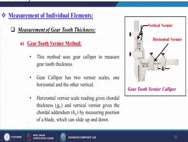
Now measurement of the individual elements like measurement gear tooth thickness here tooth vernier method first one this method uses gear caliper to measure gear to thickness. Gear caliper has two vernier scales one horizontal and the other one is the vertical so you can see this is the horizontal vernier and this is the vertical vernier. So, this is the combinations of actually two vernier scales.
