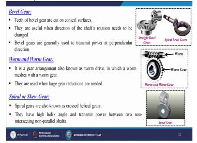
Now come to the bevel gear so teeth of bevel gear are cut on conical surfaces they are useful when direction of the shafts rotation needs to be changed. So, from these directions we are changing these directions rotation of the shaft. Bevel gears are generally used to transmit power at perpendicular direction. Worm and worm gear it is a gear arrangement also known as one drive in which a worm meshes we take worm gear so in this way this is known as the worm and this is known as the warm gear.
