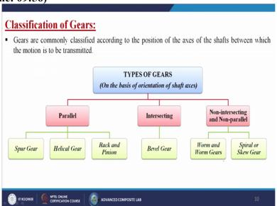
Now come to the classification of gears so generally gears are commonly classified according to the positions of the axis of the shafts between which the motion is to be transmitted. Generally there are types of gears on the basis of orientation of shaft axis if we divide so it will be three first is parallel intersecting non intersecting and non parallel. So, when you are talking about the parallel first one is called the spur gear then helical gear and the rack and pinion.
