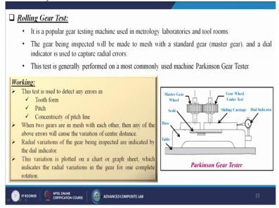
Now come to the rolling gear test it is a popular gear testing machine who used in metrology laboratories and the tool rooms the gear being inspected will be made to mesh with a standard gear generally known as the master gear and the dial indicator is used to capture the radial errors. So, simple I am having that one standard gears and then my gears will match and then there is any deflections so that means there is some kind of problems.
