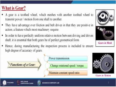
So, generally the gear is a toothed wheel which meshes with another toothed wheel to transmit power or motion from one shaft to another. So, I am having two shaft and two gears so one gear will rotate and either another will or sometimes both are rotate so, what will happen these motions will transmit to that another shaft. So, they have a advantage over frictions and belt drives in that
