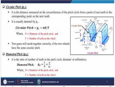
Next come to the circular pitch or in short generally we are calling it as a Pc it is the distance measured on the circumference of the pitch circle from a point of one tooth to the corresponding point on the next tooth. It is usually denoted by Pc as I told already so circular pitch Pc = PI D / T, so where D is the diameter of the pitch circle and T is the number of teeth
