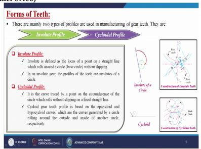
Now forms of teeth so there are mainly two types of profiles are used in manufacturing of gear teeth what are those one is called the involute profiles another one is called the cycloidal
