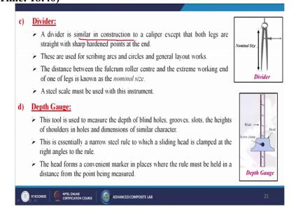
Next come to the divider a divider is similar in construction to a caliper except that both legs are straight with sharp hardened points at the end. These are used for scribing arcs and circles and general layout works. The distance between the fulcrum roller center and the extreme working end of one of legs is known as the nominal size. A steel scale must be used with this instrument.
