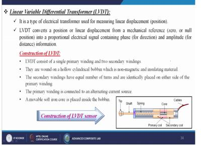
Now if we are talking about the LVDT it is a type of electrical transformer used for measuring linear displacement like position. LVDT converts a position or linear displacement from a mechanical references like zero on null position into a proportional electrical signal contacting phase for direction and amplitude for distance information. Construction of the LVDT consists of a single primary winding and two secondary windings over there.
