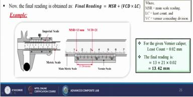
How to read a vernier caliper to read a measure from a vernier caliper first the main scale reading up to the zero of the vernier scale is noted down it will give accuracy up to the smallest divisions of the main scale. Next read the graduations or one year coinciding divisions wear to graduation lines on main and vernier scale perfectly match over there. So, in this particular case you see this is perfectly matching.
