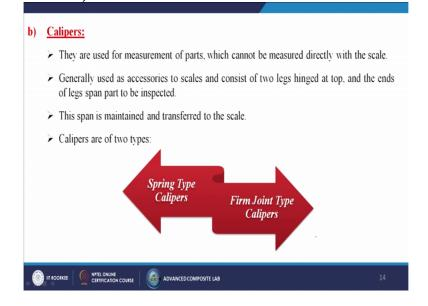
Now come to the calipers they are used for measurement of parts which cannot be measured directly with the scale. Generally used as accessories two scales and consists of two legs hinged at top and the ends of leg span part to be inspected. This span is maintained and transferred to the skill. Calipers are two types that means they are not the direct measuring tool they are the indirect measuring tool. So, one is called the spring type calipers another one is called the farm joint type calipers.
