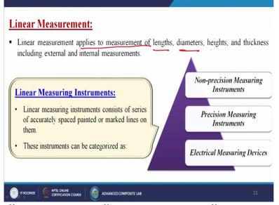
Now come to the linear measurement, linear measurement applies to measurement of lengths diameters, heights and thickness including external and the internal measurements. So, generally the linear measurement instruments are having of series of accurately spaced painted or mark on them. These instruments can be categorized as non precision measuring instruments, precision measuring instruments, electrical measuring devices. (Refer Slide Time: 11:44)
