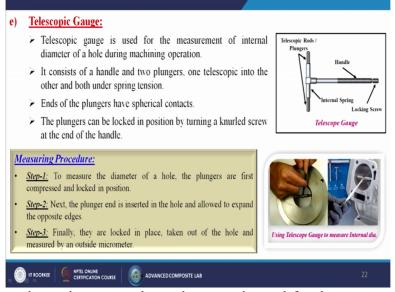
Now come to the telescopic gauge telescopic gauge is used for the measurement of internal diameter of a hole during machining operations. It consists of a handle and two plungers one telescopic into the other and both under spring tension it looks like this. These all are the telescopic rods so simple these all are the movable parts. So, inside we are putting the spring so, by this way we can measure the internal diameter of that particular part.
