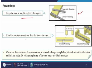
Precautions keep the rule at a right angle to the object read the measurement from directly above the rule itself so, simple from the top itself we are going to measure. Wherever there are several measurements to be made along a straight line the rule should not be raised until all are made for with each placing of the rule errors are likely to occur. (Refer Slide Time: 13:26)
