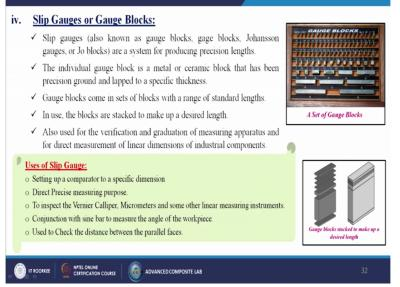
Next one is called the slip gauges or maybe the gauge block, slip gauges also known as gauge blocks gauge blocks only the spinning are different Johanssen gauges or maybe the Jo blocks are a system for producing the precision lengths. The individual gauge block is a metal or ceramic block that has been precision ground and lapped to a specific thickness. Gauge blocks come in sets of blocks with a range of standard lengths in use the blocks are stacked to make up a desired length.
