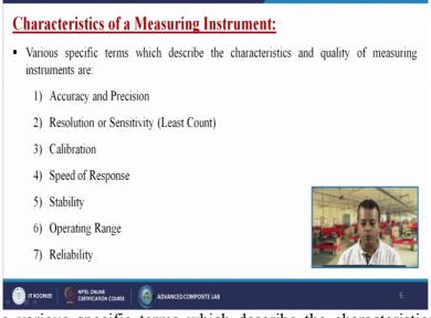
So, generally the various specific terms which describe the characteristics and quality of measuring instruments are first one is the accuracy and precision I will come one by one slowly. Second is called the resolution or sensitivity that means the least count. Third one is the calibration fourth one is the speed of response fifth is the stability sixth is the operating range and seventh is nothing but the reliability. **(Refer Slide Time: 06:20)**
