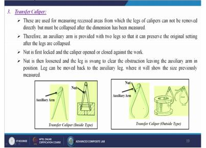
Next one is called the transfer calipers these are used for measuring recessed areas from which the legs of calipers cannot be removed directly but must be collapsed after the dimensions has been measured. Therefore an auxiliary arm is provided with two legs so that it can preserve the original setting after the legs are collapsed nut is first locked and the caliper opened or closed against the work.
