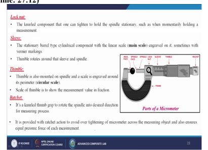
Locknut the knurled component that one can tighten to hold the spindle stationary such as when momentarily holding a measurement itself, so now in this particular case we are putting the lock nut over there so that movement of this one will be locked, sleeve the stationary barrel type cylindrical component with the linear scale main scale that is engraved on it sometimes with vernier markings. So, this is known as the sleeve.
