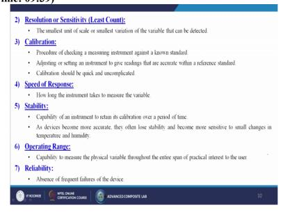
Now come to the resolution or sensitivity or maybe the least count. The smallest unit of scale or the smallest variations of the variable that can be detected, calibration procedure of checking a measuring instrument against a known standard, so suppose 1 kg so now every shop when we are going we are measuring our belongings like 1 kg but how to know that whether that is exactly 1 kg or maybe the 950 gram or maybe 1 kg 100 gram.
