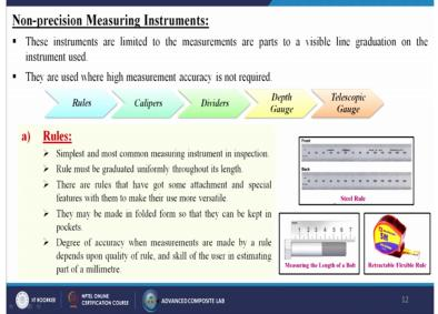
Non precision measuring instruments, these instruments are limited to the measurements are parts to a visible line graduations on the instrument used. They are used where high measurement accuracy is not required like rules, calipers, dividers depth gauges and that telescopic gauge. If we talk about the rules so simple and the most common measuring instrument in inspection, rules must be graduated uniformly throughout its length.
