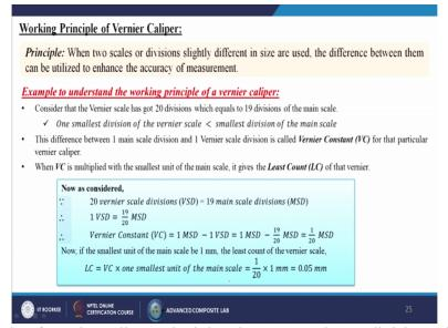
Working principle of vernier caliper principle when two scales or divisions slightly different in size are used the difference between them can be utilized to enhance the accuracy of measurement. Example to understand the working principle of a vernier caliper consider that the vernier scale has got 20 divisions which equals to the 19 divisions of the main scale, one smallest divisions of the vernier scale less the smallest division of the main scale.
