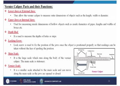
Vernier caliper parts and their functions first is called the lower jaws or may be the external jaws. So, they allow the vernier caliper to measure outer dimensions of objects such as the length width or maybe the diameter so this is the external jaws. Upper jaws or may be the internal jaws used for measuring inside dimensions of hollow objects such as inside diameters of pipes, lengths and widths of the boxes.
