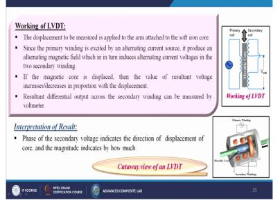
Now working of the LVDT the displacement to be measured is applied to the arm attached to the soft iron core since the primary winding is excited by an alternating current source it produces an alternating magnetic field which in turn induced alternating current voltages in the two secondary windings if the magnetic core is displaced then the value of resultant voltage increases or decreases in proportion with the displacement itself.
