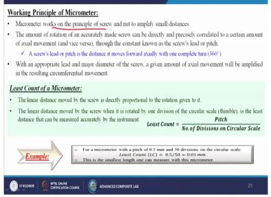
Now working principle of the micrometer: Micrometer works on the principle of screw and nut to amplify the small distances the amount of rotation of an accurately made screw can be directly and precisely correlated to a certain amount of axial movement and vice versa through the constant known as the screw lead or may be the pitch. Screw lead or pitch is the distance it moves forward axially with one complete turn that is 360 degree rotation.
