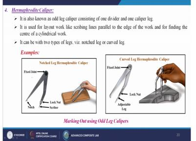
Next is that hermaphrodite caliper, it is also known as odd leg caliper consisting of one divider and one caliper leg, so here. It is used for layout work like scribing lines parallel to the edge of the work and for finding the center of a cylindrical work. It can be with two types of legs one is notched legs or maybe the curved legs. So, like this way we are having this one adjustable leg over there we are having that lock nut and then we are measuring. **(Refer Slide Time: 18:40)**
