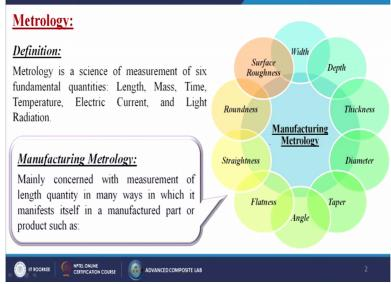
Like length, mass, time, temperature, electric current and the light radiation. So, when you are talking about the manufacturing metrology so generally it is concerned with measurement of length quantity in many ways in which it manifests itself in a manufactured part or any product such as like width, depth, thickness, diameter, taper, angle, flatness, straightness, roundness and the surface roughness.
