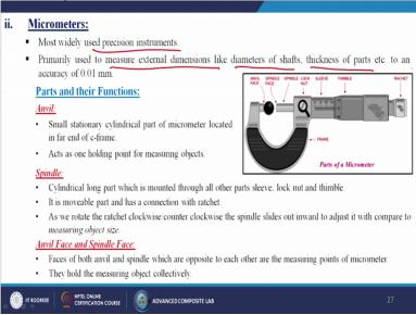
Now come to the micrometers most widely used precision instruments primarily used to measure external dimensions like dimensions of shaft's thickness of parts etcetera to an accuracy of 0.01 millimeter. Parts and their functions first one is called the anvil small
