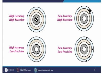
When we are; this is a bull's eye and when we are putting the bullet in a particular area within this circle so we are calling it as a high accuracy and a high precision. Then in this particular case also we are not actually putting in the center itself. We are putting somewhere else but all the bullets are together. So, in this case it is the low accuracy but the high precision because repeated values are very nearby.
