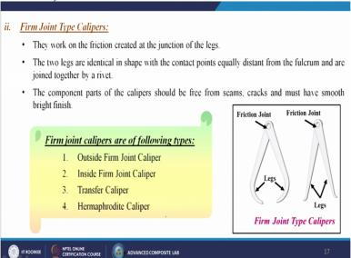
Firm joint type calipers, they work on the friction created at the junction of the legs. The two legs are identical in shape with the contact points equally distant from the fulcrum and are
