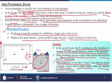
Data presentations B-scan: B scan presentations are a profile view cross-sectional of a test specimen. So in the B-scan, the time of flight travel time of the sound energy is displayed along the vertical axis and the linear position of the transducers is displayed along the horizontal axis. From the B-scan, depth of the reflector and its approved summate linear dimensions in the scan deflection direction can be determined. It almost represents a photographic type of image of the defect.
