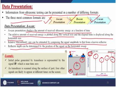
Now Data Presentations: Information from ultrasonic testing can be presented in a number of defracting or maybe the differing formats. The three most common formats are A-scan presentations, B-scan presentations and the C-scan presentations. Data presentations for A-scan: A-scan presentation displays the amount of received ultrasonic energy as a function of time. The relative amount of received energy is plotted along the vertical axis and the elapsed time is displayed along the horizontal axis.
