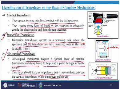
Classification of transducers on the basis of coupling mechanisms: So first is called the Contact Transducers. They appear to come into direct contact with the test specimens so in this case you are having the transducers and you are directly touching with your test surface or maybe the test specimen. They require some form of liquid or dry couplant to adequately couple the ultrasound to and from the test specimen itself.
