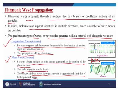
Now come to the ultrasonic wave propagation. Ultrasonic wave propagate through a medium due to vibratory or oscillating motions of its particles. In solids, molecules can support vibrations in multiple directions; hence a number of wave modes are possible, as I told already. When the atom or maybe the molecules will try to vibrate, so it will vibrate either maybe the longitudinal directions or maybe the horizontal directions or maybe in any other
