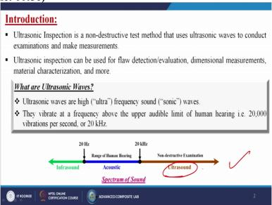
So generally the ultrasonic inspections can be used for the flaw detections or maybe the evaluations, dimensional measurements, that what is the sample weight or maybe the height or maybe the thickness, material characterizations and other more. Then what is the ultrasonic wave? Ultrasonic waves are high frequency sound waves so when I am talking about this particular chart so you can see that below 20 Hertz, generally you are calling it as a infrasound.
