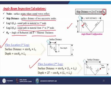
Now come to the angle beam inspection calculations. So this is the case over there. So first let us know about the nodes. Surface points where sound waves reflects, that is called the nodes. Skip distance, surface distance of two successive nodes leg1 or maybe the L1, sound path in material to first node leg2 or maybe the L2, sound path in material from first to second node Theta R, angle of refraction and T is the material thickness.
