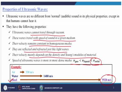
Properties of ultrasonic waves: So ultrasonic waves are no different from normal sound in its physical properties except in that humans cannot hear it. So it is beyond our audible capacity. They have the following properties. What are those? Ultrasonic waves cannot travel through the vacuum, so always it needs some media. These waves travel with speed of sound in a given medium. Their velocity remains constant in homogeneous media.
