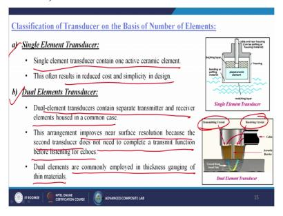
Next one is called the classification of transducers on the basis of number of elements. First one is called the Single Element Transducers. What is that? Single element transducers contain one active ceramic element. These often results in reduced cost and simplicity in design. Yes of course, if you want to increase the crystals number, so automatically the cost will increase and not only that the machine will not be or maybe the probe will not be the simple one. It will become that complex.
