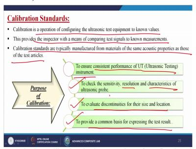
Next Calibration Standards: Calibration is the operation of configuring the ultrasonic test equipment to the known values. This provides the inspector with a means of comparing test signals to known measurements. Calibration standards are typically manufactured from materials of the same acoustic properties as those of the test articles. Purpose of the Calibrations: To ensure consistent performance of ultrasonic testing instrument to check the
