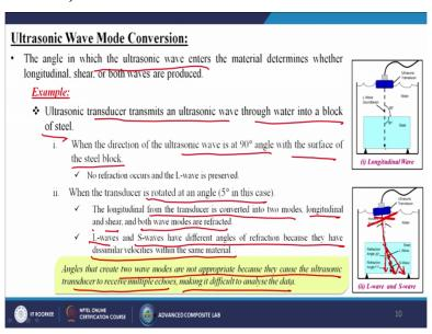
Now ultrasonic wave mode conversion: The angle in which the ultrasonic wave enters the material, determines whether the longitudinal, shear or both waves are produced. Example ultrasonic transducer transmits an ultrasonic wave through water into a block of steel. So when the direction of the ultrasonic wave is at 90 degree angle with the surface of the steel block, no reflection occurs, and the L wave is preserved.
