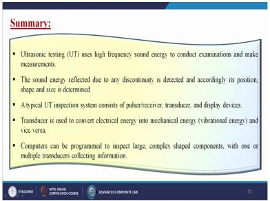
So now we have come to the last light of this particular lecture. So in summary, we can say that Ultrasonic testing uses the high frequency sound energy to conduct the examinations and make measurements. That already we have gone through. The sound energy reflected due to any discontinuity is detected and accordingly its position shape and size is determined. That also we have taken into consideration, that how we can calculate, how you can get the information.
