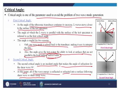
Now come to the critical angle. Critical angle is one of the parameter that used to avoid the problem of two wave mode generation. First is called the first critical angle, as the angle of the ultrasonic transducer continues to increases, L waves move closer to the surface of the test specimen. The angle at which the L wave is parallel with the surface of the test specimen is referred to as the first critical angle.
