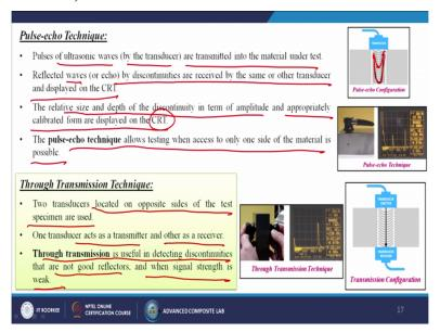
First one is called the Pulse Echo technique. So, Pulses of Ultrasonic waves by the transducers are transmitted into the material under test. Reflected waves or echo by discontinuities are received by the same or other transducers and displayed on the CRT screen. So in this case, you can see, that pulse are coming, and then it is reflecting from the bottom if there is no crack, if there is certain cracks so automatically it will be reflecting from that particular crack point.
