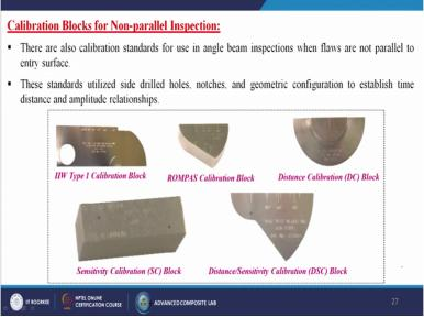
Calibration blocks for the Non parallel Inspections: There are also calibration standards for using angle beam inspections when flaws are not parallel to the entry surface. These standards utilize side drilled holes, notches, and the geometric configuration to establish time distance and amplitude relationships. Here you can see that, we have given so many examples of different calibration blocks for some kind of abnormal surfaces or maybe the irregular surfaces.
