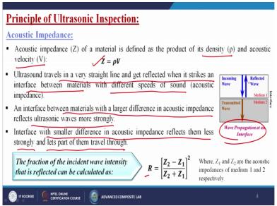
Now Principle of the Ultrasonic Inspections: First is called the Acoustic impedance. What is that? Acoustic impedance Z of a material is defined as the product of its density Rho and the acoustic velocity V. So simple generally we are calling acoustic impedance Z is equal to Rho and V. Ultrasound travels in a very straight line and get reflected when it strikes an interface between materials with different speeds of sound acoustic impedance.
