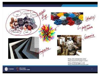
Now on your screen you can see different classes or different types of engineering materials, the first category that we have highlighted here are the metals or the alloys, you can see it is clearly written the names are given metal or alloys. So you can see here aluminium, brass, cast iron, copper, steel, bronze, metal sludge. So all these fall under the category of metals or alloys.
