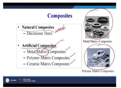
We can purpose the use of the ceramics, then finally we come to another category that is composite, now composites can be natural composities, one of the natural composite that is wood, then there are man made of synthetic composite, such synthetic composites are 3 types, metal matrix composites, polymer matrix composites and ceramic matrix composites. Few examples are given for metal matrix composites.
