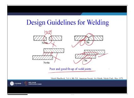
Now these are the design guidelines for welding this is not recommended lot of distance between the 2. So, this is better joint preparation here also lot of gap, so may be a better gap management here. So, this is recommended and these 2 are not recommended poor and good fit-up of the weld joints. So, this also not only this we have seen a lot many designs or design modifications suggested by the engineers and scientist which help us to make good joints.
