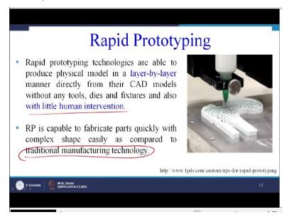
So, rapid pro-typing technologies are able to produce physical model in a layer-by-layer manner directly from the CAD models without any tools, dies and fixtures and also with little human intervention. So most of the rapid prototyping processes are automatic in nature, RP is capable to fabricate parts quickly with complex shapes easily as compared to the traditional manufacturing technology.
