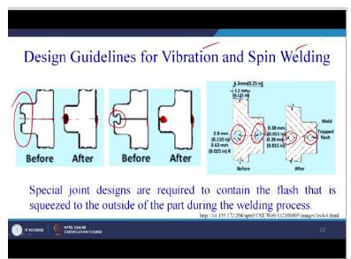
Now these are the design guidelines for vibration and spin welding all of us know that when we are joining the 2 plastic parts. And in the previous slide we have seen that there is a melting of the plastic at the interface. So, there is a tendency of this plastic to move out as a flash when it is in the molten state and when we apply or certain amount of pressure. So, when under that pressure the molten plastic may come out at the edge and form of flash.
