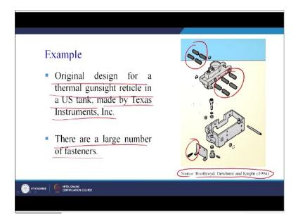
So, this case study taken from that book Boothroyd Dewhurst Knight published in 1994 product design for manufacturing and assembly. So, example is this is original design for a thermal gunsight reticle in US tank made by Texas Instruments. There are large number of fasteners here we can see large number of fasteners are there.
