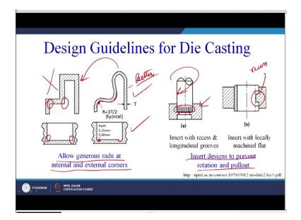
So, one of the guidelines is allow the generous radii at internal and external corner, so we can see here there are sharp corners and here it is a rounded corner again sharp corner rounded corner. So, this is may be a better design as compared to this design, so this is not recommended for die casting this is recommended for die casting. Similarly here also sharp corners are there, here there are radii provided a better design for the die casting point of view.
