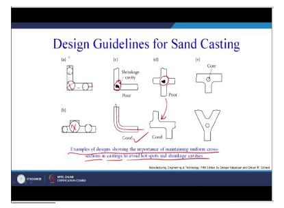
Now these are the may be once we have selected the process, for example we selecting casting process then this type of information is available as you can see on your screen. So, the design guidelines for sand casting, so we have seen these are the examples of designs showing the importance of maintaining uniform cross-sections in casting to avoid hot spots and shrinkage cavities this is the shrinkage cavity here shrinkage cavity here.
