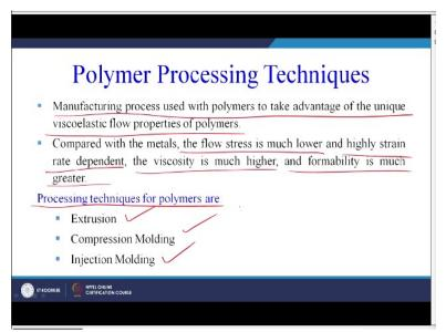
Now compared with metals the flow stresses much lower highly strain rate dependent the viscosity is much higher and formability is much greater. So, this is basically different techniques are used extrusion, compression molding and injection molding.
