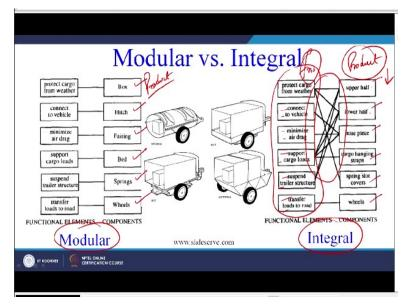
So, we will not be able to going to the details of this but in modular architecture each part box, hitch, fairing, bed, springs, wheels or may be independently satisfying a particular function or their satisfying the functional requirement independently, whereas in case of a integral we can see that there is a inter-relationship among the various parts the upper half, lower half, nose piece, cargo, hanging straps, spring slot covers, wheels.
