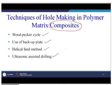
Then we have also discussed in our course the techniques for hole making in polymer matrix composites. So, we have seen there are different types of materials may be metals, ceramics, polymers, composites. So, for composites we have seen there are number of problems associated,
