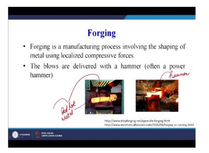
And forging is a manufacturing process involving the shaping of metals using localised compressive forces, so we might have seen the black smith they produce a fan hooks or to other product day to day product. So this is fan hooks are an important example of the forging process. The blows are delivered with hammer often with a power hammer. So forging also has got different types of modifications or variant we may have hand forging, we may have a machine forging, squeeze forging, press forging.
