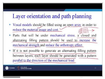
So, layer orientation and path planning visual models should be filled using an open array in order to reduce the material usage and cost. So visual model should be filled using an open array in order to reduce the material usage and cost. Now there are open array we can select the fill density in our model as per our choice. So, may be many cases we just want to see that how the product will look like?.
