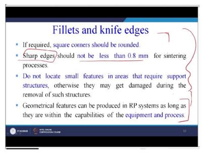
If required square corners should be rounded, so we must avoid the use of square corners and we must try to round them off. Sharp edges should not be less than 0.8 millimetre for sintering processes. So sharp edges must be avoided, range is also given should not be less than 0.8 millimetre do not locate small features in areas that require support structures. Now in many cases I must address this support structure issue here.
