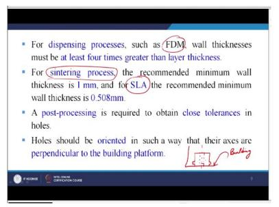
Wall thickness is I have already told must be at least 4 times greater than the layer thickness. So, whatever layer thickness we have decided and if you go back to the previous slide we can see it is already there 0.8 millimetre multiplied by 4 you will somewhere get 0.72 millimetre, so 4 times the wall thickness. So, layer thickness must be 1/4th of the minimum wall thickness or in the next slide we have written that minimum wall thickness must be 4 times the layer thickness.
