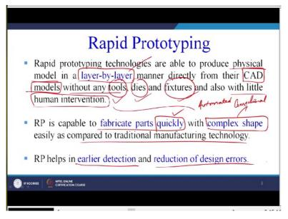
So, this is very important physical model in a layer by layer this is very important and already highlighted. We make a prototype layer by layer, layer on top of the other layer directly from their CAD models, as I have already highlighted with the development in our computational systems. CAD models are being developed for most of the 3 dimensional objects and then these models can easily be used to create a prototype layer by layer.
