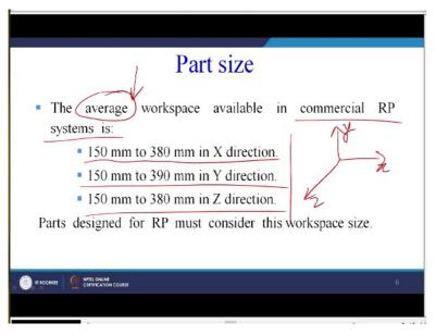
So, I must say the word average here is very very important because as I have already told that 70 to 80 different process is fall under the broad umbrella of rapid prototyping. So, the average work space available in commercial RP system is, so this is generally it is not specific to any one rapid prototyping strategy or process it is the general guideline that we can have 150 millimetre to 380 millimetre in X direction, 150 to 390 Y and 150 to 380 in Z direction.
