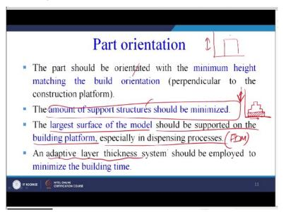
The part should be oriented with the minimum height matching the build orientation perpendicular to the construction platform. So again suppose this is the construction platform which is going to move up and down, so we have to the part should be oriented with the minimum height matching the build orientation. So minimum height we have to see, what is the minimum height and it must match with the build orientation.
