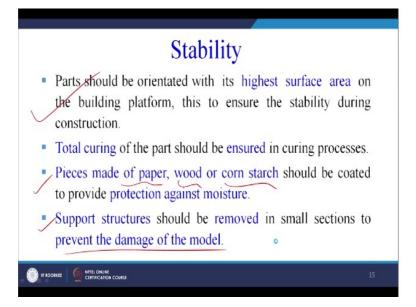
Now stability part should be oriented with higher surface area on the building platform, this is to ensure the stability during construction already discussed I have explained it with the help of a diagram total curing of the part should be ensured in the curing process very important because the parts will polymerise and solidify once the curing is complete, so we must ensure complete curing of our prototyped parts.
