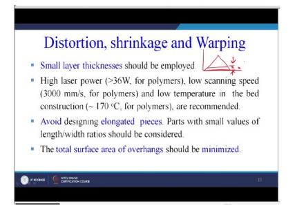
So, how to overcome that small layer thickness is should be employed, so as we have already taken an example again I am making the same part. So this thickness X must be less, so small layer thicknesses should be employed, high laser power maybe greater than 36 watt for polymers low scanning speed 3000 millimetre per second for polymer and low temperature in the bed construction that is approximately equal to 170 degree centigrade of polymers are recommended very good guideline for the polymers.
