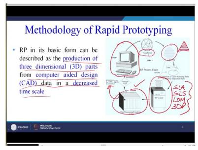
So, the rapid prototyping in its basic form can be described as the production 3 dimensional physical part from computer aided design data in the decreased time scale. So, time is less CAD model is required we have a rapid prototyping system which will create the CAD model into a physical object or 3 dimensional CAD model into a physical object. So, we can see here step by step, first step is a CAD model of the part.
