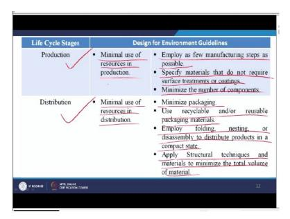
Now at the production stage we can say minimal use of resources in production, employee as few manufacturing steps as possible. Specify materials that do not require surface treatments or coatings, minimise the number of components in design for a assembly also we say use the modular design. Similarly distribution minimal use of resources in distribution, minimise the packaging, use recyclable or reusable packaging materials.
