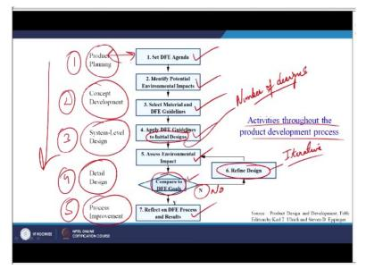
So, we can see all the 7 steps are now reflected in a flowchart, so first is set the DFE Agenda which we have already seen identify the potential environmental impacts, select materials and DFE guidelines. Apply DFE guidelines on initial designs very very important because we need to have a number of initial designs. And then we have to finalize that which design is going to help us.
