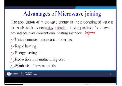
Now what are the advantages of the microwave joining, the application of microwave energy in the processing of various materials such as ceramics, metals and composites offers several advantages over conventional heating methods. So they can be use for ceramics, metals and composites or we can also say polymer based composites what are the advantages unique microstructure.
