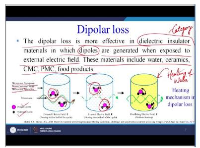
You can see the dipolar loss is more effective in dielectric insulator, so this is again a category of a material, some materials will dielectric insulators in which dipoles are generated when exposed to external electric field. So dipoles we can see the dipoles here in the diagram are generated when exposed to the external electric field. These materials include water ceramic, ceramic matrix composites, polymer composites and the food products.
