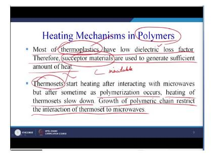
So most of the thermoplastics have low dielectric loss factor, therefore susceptor materials are used to generate sufficient amount of heat. So we can see here the depending upon the dielectric properties of the polymers we may not be able to produce or sufficient amount of heat and therefore the need of the susceptor materials becomes inevitable. So we are able to produce sufficient heat in case of polymers by using the susceptor materials.
