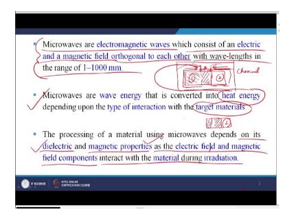
Now microwaves what are microwaves now, microwaves are electromagnetic waves which consist of an electric and magnetic field orthogonal to each other with wavelengths in the range of 1-1000 millimetre. So this clearly gives us an idea that what microwaves actually are? and these are the same microwaves that we use for heating or cooking of our food in our domestic ovens or the domestic microwave ovens.
