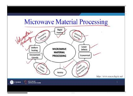
There are number of advantages, so already I have highlighted this part which I am again writing that it is an important characteristics of microwave that it leads to volumetric heating. So the everywhere in the product or the component or the joint that we are making the temperature will be more or less constant. So which is an example of the volumetric heating, so when the volumetric heating takes place the heating process is fast, uniform heating.
