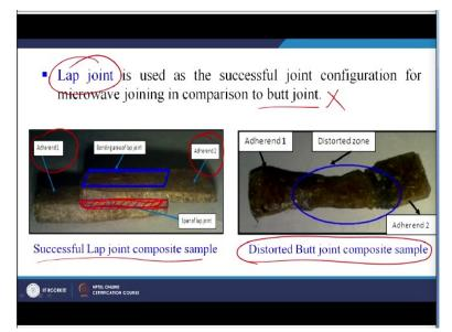
Now this is just one case study that we have done at IIT Roorkee, a lap joint is used as a successful joint configuration for microwave joining in comparison to butt joint. So this is maybe lap joint is more suitable as compared to a butt joint in case of microwave joining. So, this is a joint which was formed using the microwave energy and this is adherend number one, this is a adherend number 2. So, 2 adherend joints like this in this case it is like this.
