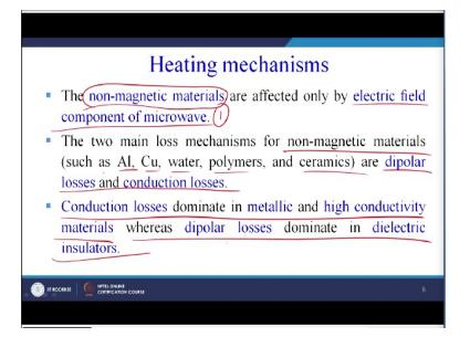
We have seen that the different types of materials will behave differently on exposure to the microwave radiation. So, the non magnetic materials let us take the first case the non-magnetic materials are affected only by the electric field component of the microwave. So, in the very beginning maybe 2 slides before this we have already seen that the electromagnetic radiation or the microwave radiation consists of 2 components electric component and the magnetic components.
