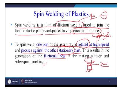
Now spin welding is a form of friction welding so already the hint is there that what is the process which is used for joining of metals. Now spin welding is a form of friction welding used to join the thermoplastic parts work pieces having circular joint line. So this is one important application area for which the spin welding of plastics can be done.
