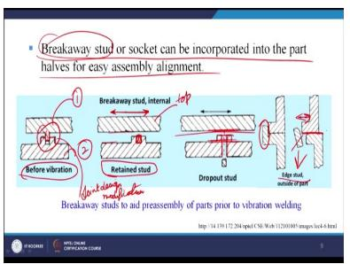
Now 2 parts have to be aligned, this is the first plastic part, second plastic part they have to be aligned. So, this type of an arrangement design modification can be done that they are aligned properly. So this is the motion or the vibration which is given to the top part which have to be welded to this part.
