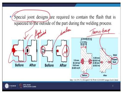
We will see with the help of diagram are required to contain the flash that is squeezed to the outside of the part during the vibration or the spin welding process. So, we have seen I will go back again to the previous slide and see that this is the area where the flash has formed. And this is completely undesirable because it adds another finishing operation once the product is ready.
