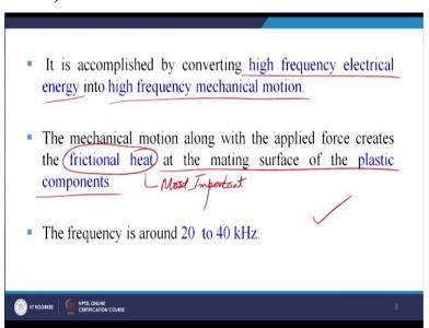
It is accomplished by converting high frequency electrical energy given to the horn into the high frequency mechanical motion. So, the 2 parts rub against each other under the applied force, so the mechanical motion along with a applied force creates a frictional heat. Already I have discussed this word, so this is the most important source of heat in case of our ultrasonic welding, so this is most important.
