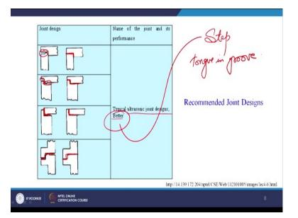
So, these are the recommended joint designs for ultrasonic welding of plastics we can see what are the types of joints you can see here, this is the joint we are getting after ultrasonic welding maybe it can be called a L type joint. Then this is another we can have joint line here and a joint line here which is final form this shown like this you can see then again we can have a joint line here and a joint line here which is shown here the 2 parts are joined.
