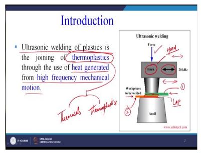
So, let us see this is a very simple diagram on your screen here we can see this is a horn if it is not clear I can write it again. This is the horn, so this is given a vibration ultrasonic frequency we can see the force is applied here already it is shown there is a force here. So, basically this load will ensure the 2 parts are in contact. Now what are the parts that we are joining this green portion is our first part and the orange portion is our second part.
