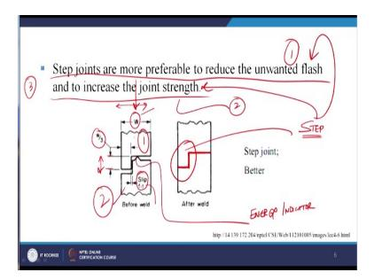
Now here we can see the step joints, this is the third guideline, so if we go back to the previous slide and try to see what are the guidelines we have seen. There must be no warpage or distortion in the surfaces that you want to join, secondly energy indicators are little molded portions at the surface during the molding stage can help to increase the frictional heat as well as the melting rate.
