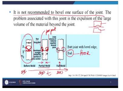
So, it is not recommended to bevel 1 surface of the joint, another important guideline this is related in fact to the first guideline that we have seen. That when we have 2 parts with warpage or distortion we may not get a good joint. Similarly if we in this, this is an higher order case of this type of joining or this type of problem. Here we have bevel here you can see, so it is not recommended to bevel 1 surface of the joint.
