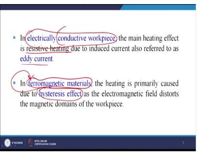
Now in electrically conductive workpiece this is just simply trying to explain the mechanism that if the workpiece is electrically conductive how the joint will be formed. And if the workpiece is ferromagnetic how the joint will be formed, let us try to understand that with these 2 sentences in electrically conductive workpiece the main heating effect is resistive heating due to induced current which is also referred to as the eddy current.
