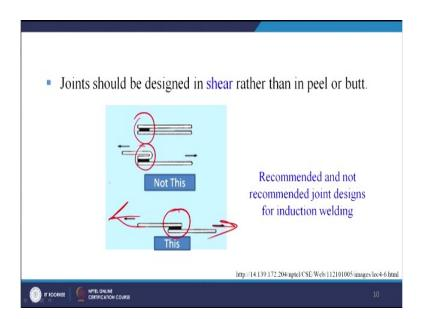
Now this is another design guideline, joints should be designed in shear rather than in peel or butt. So, whenever we are designing a joint which has to be made by the induction welding process especially for plastics they maybe designed for shear. Now this is the design for shear load ejecting in this direction and in this direction whereas the other 2 joints that we see here these 2 joints these are not in shear maybe they are in peel or butt mode.
