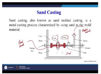
So we are not going to go into the design of the riser or the design of a core or the material required of the shape of the riser or how the riser must be placed in the casting process. So for that there are course which are already available. So in casting process what is primarily done is that we have a mild which we can see that we have a mold cavity which is here. This is my mold cavity.
