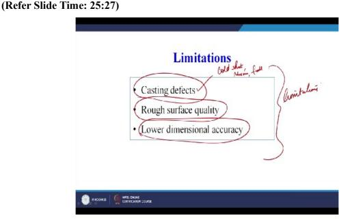
There are number of casting defect such as we can have a cold shut, we can have a miss run, we can have drop or fall, there can be different types, sometimes the metal flow that are very
