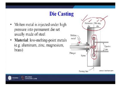
And we can avoid all these limitations of the casting process by proper optimisation of the various parameter that define the casting process. So this is one process let us now take the advanced version of the sand casting process that is the die casting processing, in die casting processing the molten metal is injected under high pressure into the permanent die set usually made of steel.
