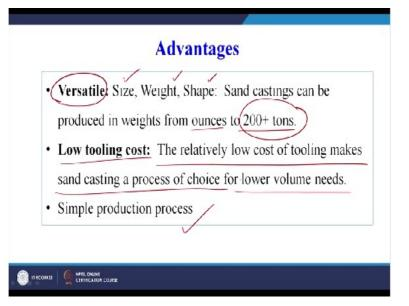
We will also understand the application areas also, but what are the advantages, now sand casting is a very very versatile process, so versatile means that if your product design changes what you can do, you only need to change the pattern which is going to create a mold cavity. So once you change the design of a pattern you can take it to the sand mold, the sand can be reused although with certain additives and modifications.
