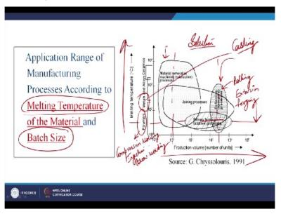
So this is showing the selection of a process based on 2 criteria, the criteria are the melting temperature of the material and the batch size. So the batch size is on x axis and the melting temperature is on y axis and this classification we have seen yesterday that we can classify the processes into 6 basic categories. So we are again revising that once we have to select a process we need to understand that which particular process is applicable under which type of circumstances.
