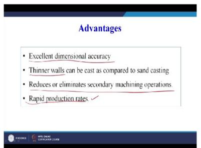
What are the advantages which has got you have seen in sand casting dimensional accuracy is not that good, but in case of die casting the dimensional accuracy that we can achieve is very very good, even thinner walls can be cost as compare to the sand casting. So in sand casting imitation is on the wall thickness. So thinner walls cannot be cast because of the problems associated with the casting defects.
