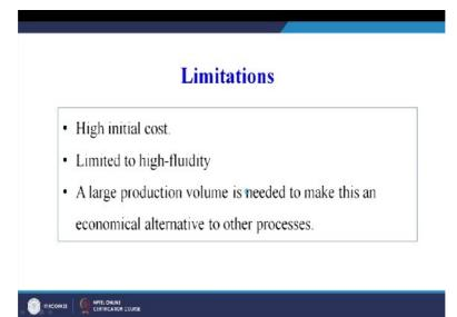
The cost of set up the cost of the machine is high in case of die casting limited to high fluidity metals only, the large production volume is needed to make this an economical alternative to other processes. So we cannot use die casting only for making 10 products or 20 products or 50 products we can use sand casting for that, but die casting is not advisable for small batch size or small number of product.
