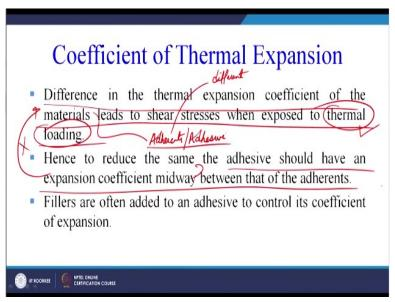
Difference in the thermal expansion coefficient of the materials lead to shear stresses when exposed to thermal loading. Now the different materials in this case maybe we can take an example of the adherents, so we have the adherents and we have the adhesive. So 2 different materials are there and in some cases the adherents may also be different, so your adherents are different your adhesive is a different material.
