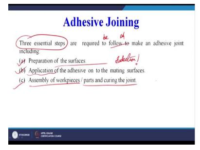
Now adhesive joining essentially requires 3 steps which also we have covered in the previous class. So, these are required to follow required maybe we can say to be followed to make an adhesive joint. Now these are the step involved first one is the preparation of the surfaces, so we have to see that the surface that we are going to join together must be adequately ready for making a joint.
