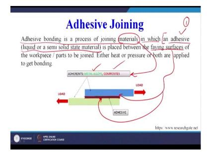
Adhesive joining is a process of joining materials the materials which are already mentioned here we can see the materials can be metals, alloys, composites, plastics, wood different types materials. So, adhesive joining is a process of joining material in which an adhesive which can be a liquid or a semi-solid material, this is adhesive 1K ingredient for ensuring the adhesive joining is placed between the faying surfaces.
