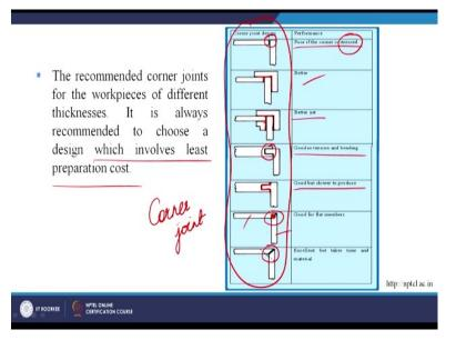
Now this is the recommended corner joints we can see 3 types of joint configurations we have seen. First one is related to the butt type of joint, second one is related to the lap type of joint and third one is related to the corner type of joint. So, the recommended corner joints for the workpieces of different thicknesses it is always recommended to choose a design which involves least preparation cost.
