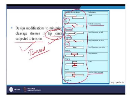
So, here we can see design modifications to minimize cleavage stresses in lap joint subjected to tension. So, here the joint configurations also fixed it is lap joint, the loading is also fixed which is tension. So, lap joints under tension what are the possibilities available with us when we have to make our product we have to ensure that the 2 parts which are going to be used in my product will be used under the lap joint configuration and the maximum loading will be under tension.
