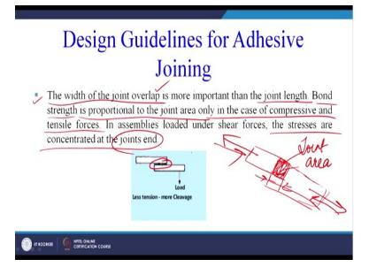
Now the width of the joint overlap, this is an important guideline, the previous one was that when we are designing the product we must ensure that what type of loading is going to come on the product. And if we are using the adhesive joining what type of loads it can bear or resist easily and what type of loading are detrimental to the performance of the product. So, we have seen peel and cleavage stresses are somehow going to be having an adverse effect on the product.
