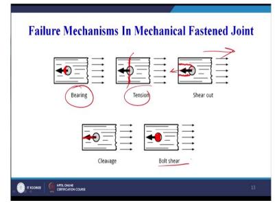
Now failure mechanisms in mechanical fastened joints we can see here, we can have bearing type of failure under tension. This is the type of failure which may take place, shearing out we are applying the load in this direction and this may shear out in this direction. Then cleavage can be formed it is shown here, it is a bolt shear can also take place, the bolt may also fail, the workpiece may fail or the bolt may also fail in some cases.
