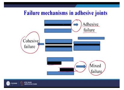
Now these are the failure mechanisms likely we are going into the depth now, these can be adhesive can fail, adhesive failure. There can be mixed failure this can get de-bonded from here and the adhesive has also failed from here then there is a cohesive failure here. So, different type of failure may take place when the product is loaded under the different types of loading environments it can be compressive load, it can be tensile load here we are showing tensile only.
