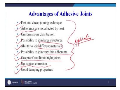
If you have understood the adhesive joining it will be easier to understand fast and cheap joining technique, adherents are not affected by heat maybe adherents are not effective. But if lot of heat is there the adhesive may get affected by the heat if in service you find lot of heat. Uniform stress distribution, no stress concentration is there uniformly the stress is distributed over the whole adhesive area, possibility to join large structures, ability to join different materials.
