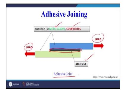
Again this is explained here we can use metal alloys also that adherents, composites can be used. This is the load that is being applied, this is the joint a black portion and this is the adhesive which has been used, this is the adhesive joint. So, we can see very easy process, very simple process, no expertise is required maybe little bit of training can help you to make the adhesive joints.
