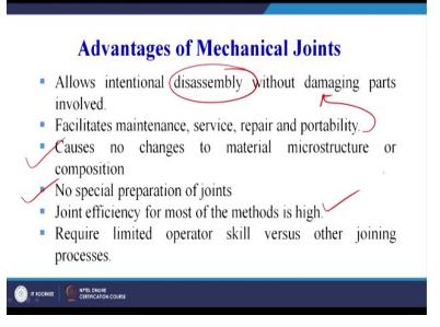
This allows intentional disassembly without damaging the parts involved, this is as we have seen it is not a permanent joining techniques. So, we can disassemble the structures also where mechanical joints or mechanical fasteners used. Facilitates maintenance, service, repair and portability which is a direct reflection of the first point. If you can disassemble your structure you can easily do maintenance service repair and portability.
