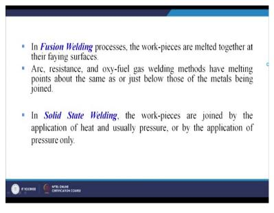
So, fusion welding, in fusion welding processes the workpieces are melted together at their faying surfaces. Arc welding resistance and oxy-fuel gas welding methods have melting points above the same as or just below those of the metals being joined. In so we will heat the metal, we will try to melt the metal and then fuse the metal together to form the joint, examples are given.
