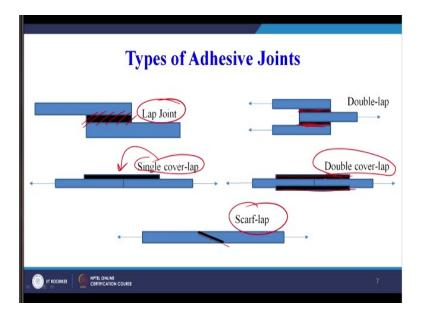
Now different types of adhesive joints can be there one is a lap joint, this is the joint area or the joint interface. Then double lap this is one adhesive bonding, this is second then double cover lap joint we can see this is double cover is there, this is the overlap area here. Then the scarf we can see this is a scarf joint, this is single cover lap, cover lap is on one side only here it is on 2 side.
