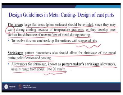
Now there are other guidelines also the design guidelines in metal casting that are related to the flat areas. Large flat areas or the plain surfaces should be avoided since they may warp one defect warpage, change in shape during the cooling because of the temperature gradients or they develop poor surface finish because of the uneven flow of the metal during pouring.
