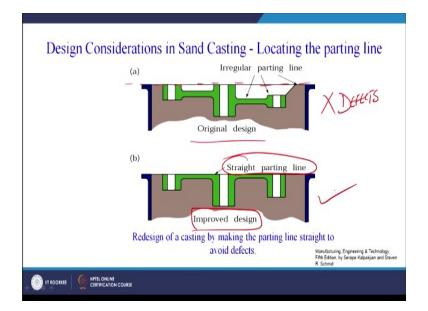
So, we have seen the parting line, now this is basically what is the parting line, so it must be straight it must not be contoured. This is the original design, so this is a straight parting line which is good this is a improved design it must be straight but here it is not straight in this case. This is a original design it can be improved by making the parting line like this redesign of a casting by making the parting line straight to avoid the defects.
