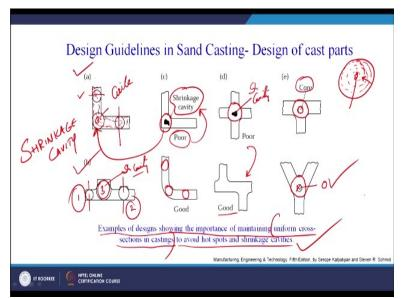
Then this is again related to the design of the parts, now this is 1 channel A, 1 product this has a tendency to form a shrinkage cavity if you can read it I will write here. It is shrinkage cavity and it can be easily located that where the shrinkage cavity will be formed why because here there is more metal because of this circle inscribed circle at the different cross-sections of the product design or the product geometry, we can see that where we can fit in the biggest circle.
