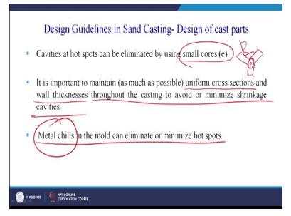
Now cavities at hotspots can be eliminated by using small cores that we have seen in the diagram towards the right hand side where a y channel was shown at the center we can have channel sorry channel like this was shown. So, here there are chances, so we can put a core here, so that we can these are change the design modification to avoid the shrinkage cavities, it is important to maintain as much as possible again this guideline is coming.
