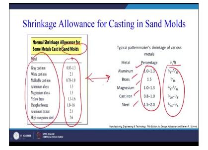
Now what we have already discussed the shrinkage allowance for casting in sand mold this is given here, this has been taken from manufacturing and technology by Kalpakjian and Schmid. So, normal shrinkage allowance for some metals casting the sand molds, so we are studying sand molding, so what is a shrinkage metal sorry the shrinkage allowance to be given for different metals this is long list of metals given here and this is a percentage of shrinkage allowance that must be given.
