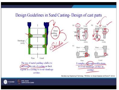
Now here we can see this is a metal chill here design guidelines in sand casting for the cast parts, now here we can see here you if you make a circle there are chances or formation of shrinkage cavity similar is the case here also. So, location can be easily identified, now how it can be avoided we can accelerate the rate of cooling why the shrinkage cavities forming or the hotspots because of the slower rate of cooling.
