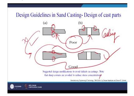
Now here we can see this is a sharp corner here again here, so what can be done the process if it is possible then you can may give a fillet here and here also instead of sharp transition we can have a gradual transition. So, both of these are poor product designs from the casting point of view and both of these are good designs from the casting point of view. So, sometimes it may not be possible for us to do these type of modifications from here to here may not be possible why?.
