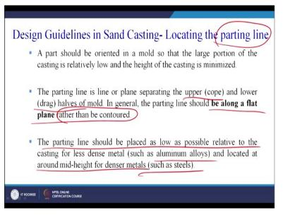
So, this is the last part we have already seen what is the parting line, so this is guideline related to the parting line. A part should be oriented in the mold so that the large portion of the casting is relatively low and the height of the casting is minimized. So, we have to decide that how much of the casting has to be in the cope part and how much has to be in the drag part.
