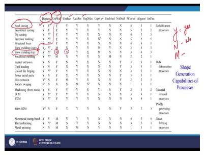
So, this is the table that I was referring to, now let us quickly see for example our sand casting process depress first column in 1 direction it can produce as well as in the multiple directions also it can produce. Uniform wall thickness is achievable by sand casting uniform section is axis of rotation is also yes, so Y means yes here and N means no. Similarly let us now take blow molding, so let us take another example that is blow molding.
