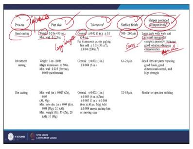
And here we have that table, so we can see here the process we are talking about the process capabilities in our session today, what are the capabilities part size, capability in terms of producing the part size, tolerances which are achievable, surface finish, shapes that can be produced competitively very very important competitively.
