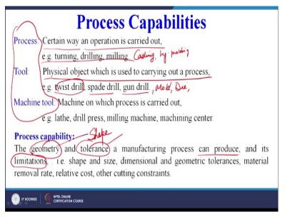
A process is a certain way an operation is carried out, for examples are given turning, drilling, milling you can have other examples for shaping the parts, you can have casting, you can have injection molding for plastics any process. So in the process it is a certain way, method, procedure in which it is being carried out, what is a tool. A tool is a physical object which is use
