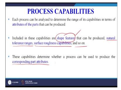
So, let us now quickly see that process capabilities that with example maybe for the specifically we will focus on the shapes and then try to see that which process can produce which type of shapes. So, each process can be analyzed to determine the range of it is capabilities in terms of the attributes of the parts that can be produced which already we have seen in session number 16 and 17 during week 4.
