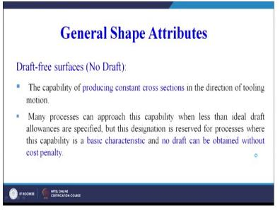
So, these are some of the general shape attributes then the draft free surfaces there is a long list of shape attributes that are that can be interrelated to the manufacturing processes. So, 1 can be draft free surface, for example there is no draft on the surface.
