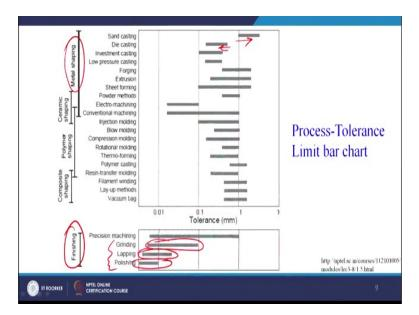
Now this is the process tolerant limit bar chart we can very easily see again there are finishing processes here which can provide better tolerance. Then there is metal shaping processes here we can see for different processes what kind of tolerance we can get. For sand casting you can see it is on the higher side whereas die casting it is comparatively lower as compared to sand casting.
