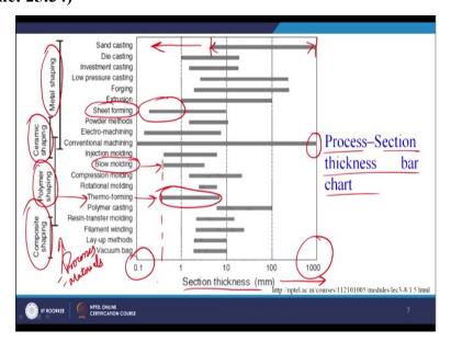
Again the processes are given here on the Y-axis metal shaping, composite shaping, polymer shaping, ceramic shaping, so the it is related to the processes. As well as you see the materials also are specified and therefore we have already discuss this classification in the first and second
