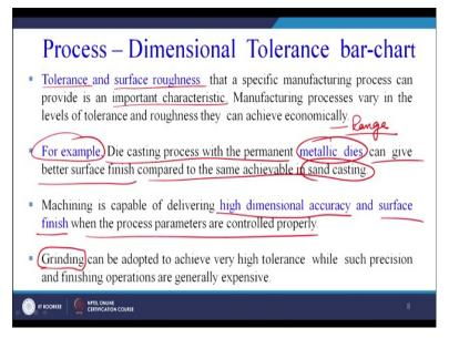
Now the next attribute is the dimensional tolerance bar chart, tolerance and surface roughness that a specific manufacturing process can provide is an important characteristics. Because this surface roughness and tolerance will directly affect the quality of the product that we are producing. So, this is an important characteristics manufacturing processes vary in the levels of tolerance and roughness they can achieve economically.
