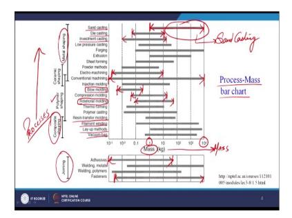
Now on your screen you can see a process mass bar chart different processes are given here and as we have seen that bulkier parts like an aeroplane can be made by joining processes also. So, the joining is also listed here as we have seen in the previous slide also and then we have sub categorization of the shaping processes. So, we have metal shaping, we have composite shaping, so obviously for composite shaping we have different processes.
