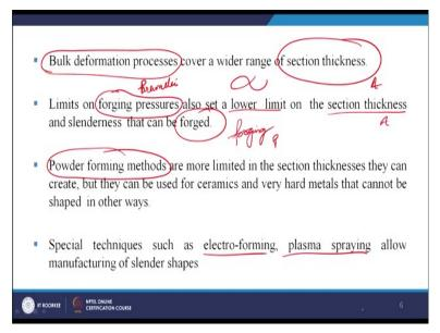
Bulk deformation processes cover a wide range of section thickness, so there another bulk deformation processes which is the process and what is our attribute that is the section thickness. So, P we have to see the relationship between the process and the attribute, so bulk deformation processes cover a wide range of section thickness another process is limits on forging pressures also set a lower limit on the section thickness and slenderness that can be forged.
