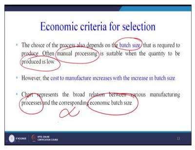
The choice of the process also depends on the batch size, the number of parts to be produced that is required to produce often manual processing is suitable when the quantity to be produced is low well known common sense. Manual processing when number of parts are low, however the cost of manufacture increases with the increase in batch size. So, manually if you are doing and the batch size is large the cost of manufacturing may increase.
