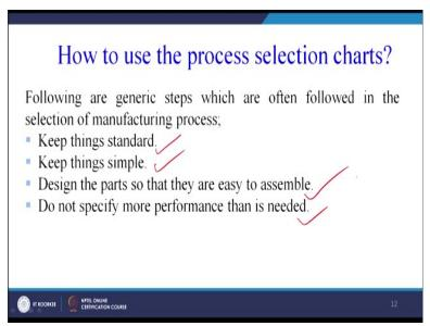
Now how to use the process selection charts just very very simple rules of thumb following are the generic steps which are often followed in the selection of the manufacturing process, keep the things standard. Keep standard means when we are designing our product we must make use of the standards keep the standards in our mind. So, that standards are set as per the manufacturing process, so therefore we know this standard can be achieved using x process.
