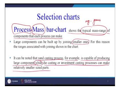
The process-mass chart as the name indicates there will be a process and there will be the change or maybe the mass or the variation in the mass that process X can be use from this much grams to this much kilogram, process Y can be used from this many kilogram to this many tons. So, this is going to be setting up a relationship between the mass and the process that for this particular mass this process is advisable.
