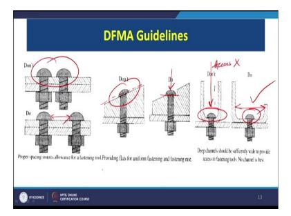
Then here we see that the proper spacing ensures allowances for fastening tool, so here you can see these are very close, the 2 fasteners. So, we can space them appropriately, so that we our fastener our holding tool or the fastening tool can easily fasten them. So, space has to be provided for fastening this is providing flats for uniform fastening and fastening ease difficult to fasten here because of the inclined surface.
