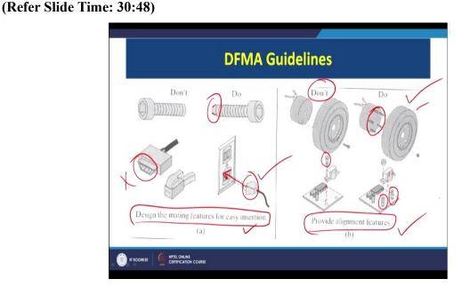
Then they here we can see that design the mating features for easy insertion is in the previous class if you remember we have seen 2 types of guidelines 1 were the handling guidelines another one were the insertion and fastening guideline. So, for easy insertion guidelines we can see a chamber is given here as I have told in the previous session also that for easy insertion a chamber can be created at the end.
