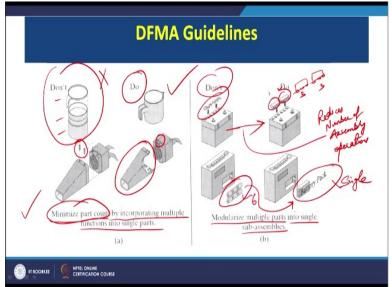
These are the guidelines which are given with examples now minimize the part count by incorporating multiple functions into single parts. Now here we can see this is do which is correct design of the part and here we see it is don't because there are 2 or 3 different parts which are assembled together. So, what is our target as per DFMA guidelines when we are designing a product, we have to minimize the part count.
