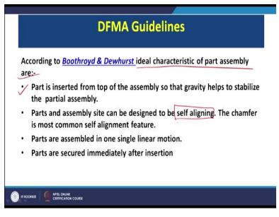
Let us try to see the part is inserted from top of the assembly so that gravity helps to stabilize the partial assembly. So, this is top down type of assembly approach part is inserted from the top of the assembly. So, that we can make use of the gravity, parts and assembly site can be designed to be self aligning, self aligning features must be taken into account, so maybe if you if we see that there are 4 protruding parts in the top plate.
