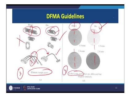
Then there other guidelines this is eliminate the tangly parts already we have seen that we have to avoid the entangling of parts when the products have to be assembled using manual assembly in our previous session. This is similar to that only, so there are parts which may entangle into each other at this point. So, we can redesign them in such a way that they do not tangle into each other.
