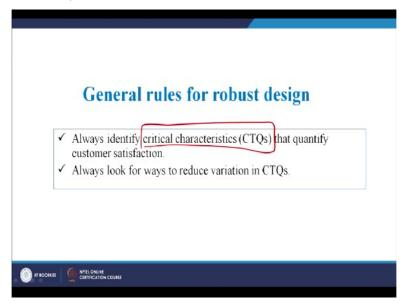
Now general use for robust design always identify the critical characteristics that quantify the customer satisfaction. So we need to identify the critical characteristics which will satisfy the customer for his needs and requirements. For example suppose I buy a new motor bike I wish that it must start all kinds of environmental condition or climatic conditions or we can say all kind of weather.
