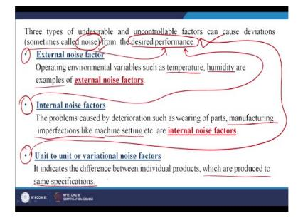
Now 3 types of undesirable and uncontrollable factors can cause deviations, in the previous slide we have seen that there are certain noise factors, which may vary form product to product. So 3 type of undesirable and uncontrollable factors can cause deviations and this is again the word noise is coming into picture here from the desired performance. Now desired performance is something which is designed into the product.
