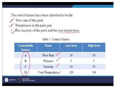
Now we have seen that what are the critical parameters that need to be taken into account as we have seen in the beginning of today's session, the control factors have been identified, so we must optimally select the flow rate, so we have seen that we have to select the parameters in order to ensure the desired performance. So that it is unaffected by the noise factor I think this sentence has been used 10 times in today's class.
