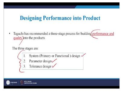
Then the tolerance design, in this step the tolerance is on the product design parameters are determined considering the loss that would be caused to society when the performance deviates from the target. And this is the most important point performance deviates from the target, this is what we have to avoid. So in this step in tolerance design step we will the tolerance is on the product design parameter determine considering that if the product deviates from the performance.
