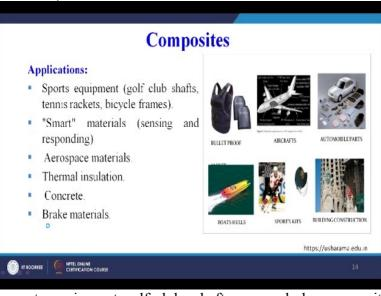
They are used in sports equipment golf clubs shafts are made by composite, tennis rackets, bicycle frames, then smart materials they are used for sensing and responding, aerospace materials they are used for lightweight application because already we have seen high strength to weight ratio is one advantage that we have with a composite materials specifically with the polymer matrix composite materials.
