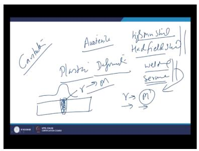
But if the joint is subjected to the impact loading during the service then it will be considered of the poor weldability otherwise the favourable weldability. There is another aspect in the deformation based or deformation assisted phase transformations like there few categories of the steels where the met steel is primarily having the austenite at room temperature, like in high manganese steels or had filled steel.
