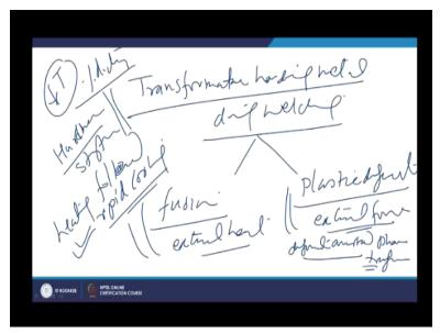
So in which way the material will be behaving means the transformation hardening metals will be behaving during the welding, we know that the welding broadly we can group under the two categories where the fusion is realized through the application of the external heat or very controlled plastic deformation is realized at the faying surfaces through the use of the external force.
