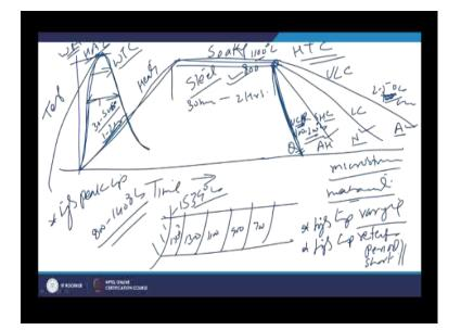
Basically heat treatment condition of the metal in which the welding is being performed, now we will try to see very closely the way by which the welding will be affecting the characteristics of the transformation hardening material say in X axis we have the time and in the y-axis we have the temperature. So if we try to understand the way by which weld thermal cycle shows the variation in temperature as a function of time.
