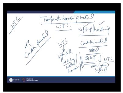
So now if we see the way by which we can understand the weld thermal cycle and it is effect on the weld joint characteristics of the transformation hardening materials. So transformation hardening metals so due to the weld thermal cycle experienced by the weld metal and the heat affected zone there can be softening or hardening as for the condition of the metal which is being welded which means if say for example if the steel is being welded unquenched and temper condition.
