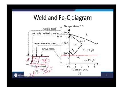
Now we will see the way by which the weld thermal cycle will be affecting are the microstructure of the steel next to the fusion boundary. So if say if we take up carbon steel is this so when the external heat is applied a part of the metal is brought to the molten state which forms the weld metal and next to that region will be experiencing the higher temperature due to the heat dissipation from the weld metal.
