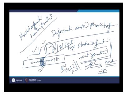
There is another aspect as far as the phase transformation hardening metals are concerned that is about the defamation assisted phase transformation. So those welding processes where huge plastic deformation is carried out for developing the required joints. So in this process lot of heat is generated and heat generated followed by the rapid cooling leads to the again formation of the hard phases in the weld zone as well as the in heat affected zone.
