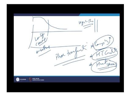
So the different zones of the same steel will be experiencing the different kind of the phase transformation and accordingly the property. So if we noticed the if we try to notice the variation in the hardness in such kind of cases then the zone next to the fusion boundary will be the hardest and then hardness will keep on decreasing. So the zone where hardness is very very high this will be experiencing the loss of toughness and this will show the tendency for cracking.
