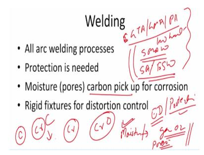
As far as the welding of the austenitic stainless steel is concerned all types of the arc welding processes can be utilized for welding of the ASS be it GTAW or GMAW or plasma arc welding. These are the processes which will be applying the low heat input. On the other hand if the high heat input process is used like SAW and electroslag welding then the high heat input will be causing more damage to the heat affected zone and likewise the shielded metal arc welding can also be used.
