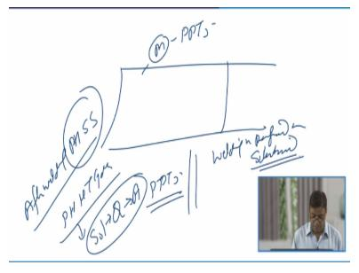
As we have seen that these steels will be gaining their strength from either development of the martensite or the development of the fine precipitates. So whenever heat is applied these precipitates will tend to get dissolved and thereby they will leading to the change in mechanical properties unfavorably. So it is always desired that after welding precipitation hardenable stainless steel are subjected to the precipitation heat treatment cycle.
