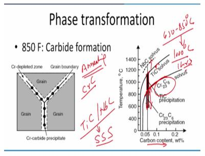
So what basically we have to see is that the different types of the carbides which are found in the austenitic stainless steels like mostly it is the formation of the chromium carbide but other carbides like titanium carbide and niobium carbides can also be formed but these will be found in case of the stabilized austenitic stainless steels. And these are formed at higher temperature.
