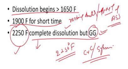
As soon as exposure is given above 1650 degree Fahrenheit, the dissolution of the sigma phase and the chromium carbide things will start and exposure at 1900 degree Fahrenheit for very short period helps in restoring the ductility and notch toughness of the ASS weld joint in the heat affected zone.
