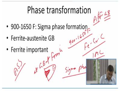
As I have said at higher temperature like say 900–1650 degree Fahrenheit. In this temperature range iron, chromium, carbon intermetallic compounds IMCs are found in form of the sigma phase formation. This sigma phase is formed at the grain boundary of the ferrite phases which are present in the ASS, the heat affected zone or in the weld metal.
