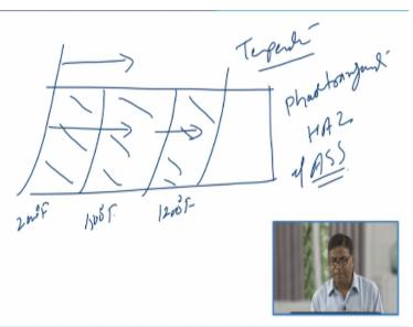
We know that when the welding of the ASS is carried out so there will be different zones which will be heated away from the fusion boundary which will be heated to the high temperatures. There will be different zones in the base metal which will be heated to the different temperatures like will be heated to the temperatures well above 2000 degree Fahrenheit. Few will be heated above 1500 degree Fahrenheit and likewise.
