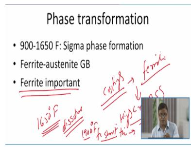
So in all those cases where the chromium content is high leading to the formation of the sufficient amount of the ferrite that will be promoting the sigma phase formation. So high chromium austenitic stainless steel will have the tendency to form the sigma phase more frequently. So here it is important that ferrite percentage in the austenite is controlled suitably so that undesirable sigma phase formation can be avoided.
