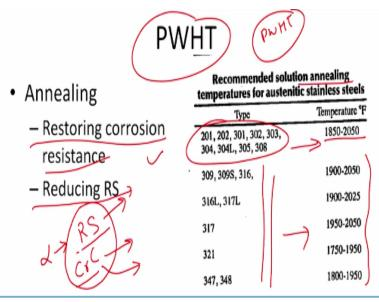
So this is how we can say that we need to be careful especially when we are performing the welding of the ASS especially with regard to the high thermal expansion coefficient because it will be trying to promote the distortion and development of the residual stresses.
