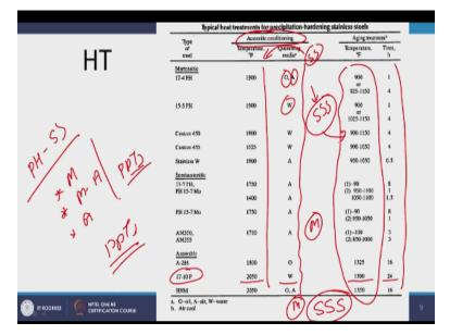
Now, in order to realize the required phases in these precipitation hardenable stainless steel whether to have the martensite or the mixture of the martensite and the austenite or the austenite or the different along with the required precipitates the different kind of the heat treatment conditions are used which of course will be involving like austenitizing by heating at higher temperature like this followed by quenching in water or oil or in air.
