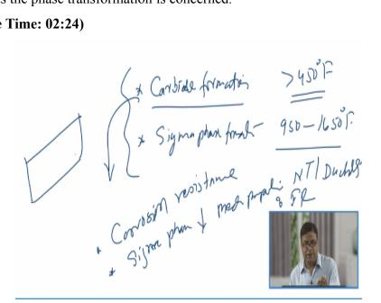
One is the chromium carbide formation. All the zones which are heated above the temperature of 450 degree Fahrenheit, they will be experiencing the carbide formation. Further at higher temperature sigma phase formation is also encountered and which is normally observed in the temperature range of 950-1650 degree Fahrenheit.
