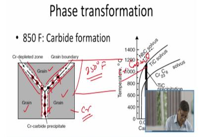
Like all the zones which are heated in the temperature range of the like say up to the 850 degree Fahrenheit, there the chromium carbide precipitation takes place. And wherever the chromium carbide precipitation takes place that zone will be experiencing the depletion of the chromium say these are the 3 different austenite grains having the chromium in solid solution.
