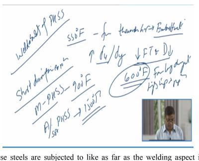
Whenever these steels are subjected to like as far as the welding aspect is concerned, weldability of the precipitation hardenable stainless steel, whenever these steels are heated above 550 degree Fahrenheit for thousands of hours it shows the embrittlement. Embrittlement will be leading to the increased or increase in yield strength and the ultimate strength.
