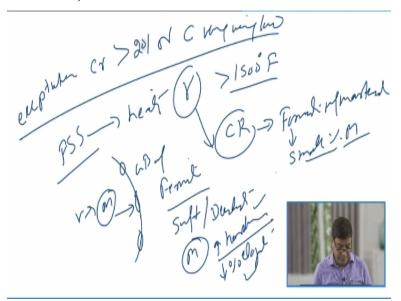
But except when the chromium content is greater than 20% or carbon content is very low usually in FSS on heating with the different grades of the ferritic stainless steels austenite is formed on heating at one or other range of the temperature. So this kind of the austenite is especially formed when the heating happens about like say greater than 1500 degree Fahrenheit.
