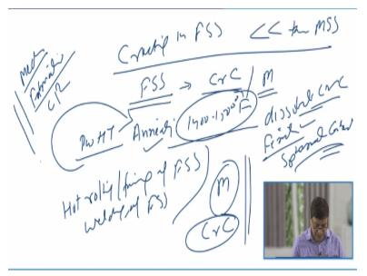
Since the fraction of the martensitic which is being formed and the hardness which is there with this kind of the stainless steels is very low so the chances for cracking in ferritic stainless steel is far less than the what we have seen in case of the martensitic stainless steel.
