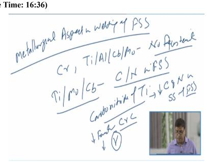
Now we will see some of the metallurgical properties related with the metallurgical aspects in welding of the ferritic stainless steel. We know that when the chromium content in these steels is high with the presence of other elements like titanium, aluminium, columbium and molybdenum, there is no austenite formation. Only ferrite is stable up to the room temperature.
