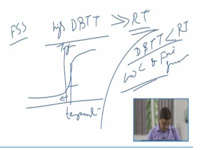
Another important aspect related with the weld joints of the ferritic stainless steel is that most of the steels have the high ductile to brittle transition temperature and we already know what this ductile brittle transition temperature is like this side we have temperature and this side we have toughness. So we know that with the drop of the temperature there is a reduction in toughness.
