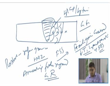
We know that the weld joints whenever it is made either by the fusion welding or by any other process different zones will be experiencing different weld thermal cycles. So zones which are very close to the fusion boundary they experience the high temperature exposure for long time. And this leads to the grain growth especially near the fusion boundary.
