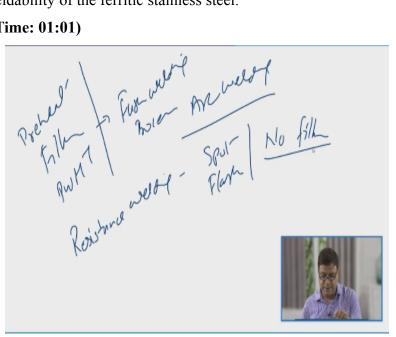
So whatever we have talked about the kind of the preheat or the filler which we have to use or the post weld heat treatment to be carried out all that was applicable for the fusion welding processes like arc welding. Now if we compare these welding processes with respect to the resistance welding processes like the spot welding and the flash butt welding. In these welding processes there is no use of the filler. No filler is used.
