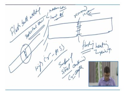
Another resistance welding process is the flash butt welding. Flash butt welding process like it is used mainly for producing the butt joints of the rods and the tubes. So here the one end is kept fixed another end is made moveable. So when the another component is brought close to the member which is to be joined with the flushing takes place. In this process of flushing heat is generated, temperature rise takes place.
