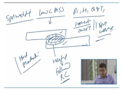
Like say as far as the spot welding is concerned, the low carbon martensitic stainless steel can be welded in all the conditions like annealed or hardened or Q & T conditions. In all those conditions whenever the plates are welded by the spot welding process like this, so we will notice that there will be partial melting and a nugget zone formation.
