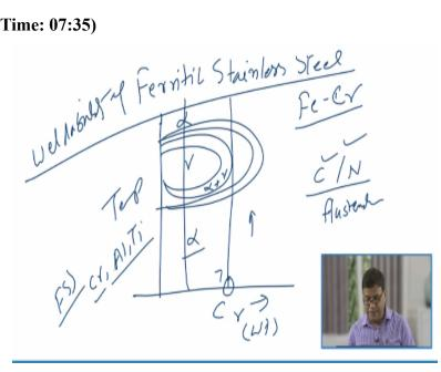
Now we will talk about the weldability of the ferritic stainless steel. Ferritic stainless steel means these are made by adding the chromium content in the iron in sufficient quantity so that the gamma loop which is found in this form like say this is the temperature scale, this is the weight percentage of the chromium. When the carbon is absent or it is very negligible so the kind of the binary phase diagram for iron and chromium shows it like this.
