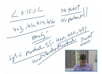
But as I have said no PWHT is needed and no major preheat requirements are there if the carbon content in the martensitic stainless steel is less than 0.15. So in the steels like 403, 410, 414 or 416 these steels can be easily spot welded without any major requirement of the preheat and the post weld heat treatment.
