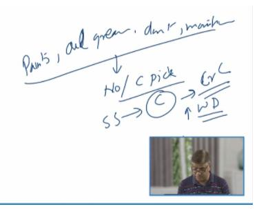
Apart from the removal of the chromium oxides effective cleaning for removing all paints, oil, grease or dust, moisture this also should be ensured so that there is no source of the hydrogen, hydrocarbons and there is no possibility for carbon pickup. Because if the stainless steel picks up the carbon during the welding it will promote the formation of the chromium carbide in the weld as well as the heat affected zone.
