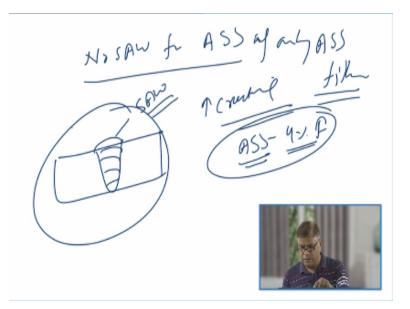
And that is why whenever possible No SAW for austenitic stainless steel welding. If only ASS filler is used because this increases the tendency for solidification cracking. If the ASS filler with the about 4% of the ferrite filler which will provide the austenitic stainless steel weld metal with the 4% ferrite in the weld zone then SAW process can be used even for the welding of the austenitic stainless steel.
