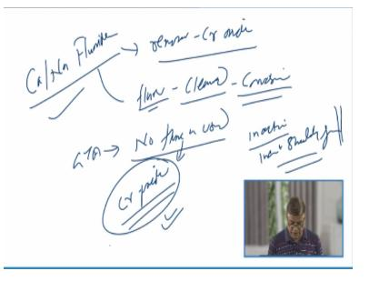
But the calcium or the sodium fluorides which are being added to remove the chromium oxides, the fluxes where such kind of chlorides are present must be cleaned because these are very corrosive in nature. So effective cleaning of such kind of the fluorides become crucial. In case of the GTA and the other gas shielding based methods, no flux is used.
