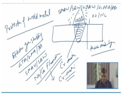
Now the protection of the weld metal is concerned, for the purpose of the protecting wave, protection is important. You know the stainless steel is subjected to the fusion welding using the different types of the welding processes like SMAW or SAW or GTAW or GMAW or PAW. In all these processes if the protection by the heat source like arc, if the protection is not proper then oxygen and nitrogen present will interact with the molten metal.
