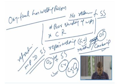
On the other hand the oxy-fuel gas welding process, this process is not recommended for welding of the stainless steels because of the poor, very poor shielding of the weld metal. So the protection of the weld metal from the atmospheric gases in case of the oxy-fuel gas welding process is limited and the heat input is also high. So that in turn reduces the cooling rate.
