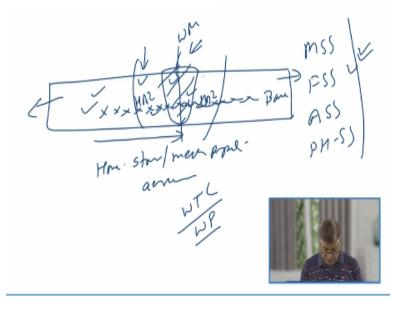
Now we will see the kind of the joint performance which is realized in case of the stainless steels since the different stainless steels like martensitic, ferritic, austenitic and precipitation hardenable stainless steels. The base and the heat affected zone HAZ and the weld metal. The properties of the joints to a great extent depends upon the homogeneity of the structure and the mechanical properties across the weld.
