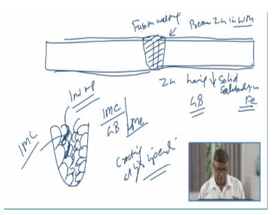
So the amount of the zinc which will be there with the steel sheet during the welding, that will bring in lot of difference in terms of the weldability like zinc coating is there both the sides of surfaces of the steel plate and when these are welded using the fusion welding processes; so in case of the fusion welding processes like we will be melting the both the faying surfaces of the both the components to be joined.
