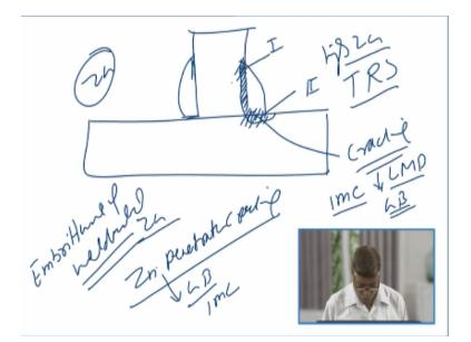
So especially when we develop the fillet joints like T- joints having the fillet welds. So what we will notice that the concentration of the zinc will be more near the root as well as in the zone 1 and zone 2 of the weld metal. And due to the high concentration of the zinc in these areas, combination with the tensile residual stresses we will get the increased cracking tendency in these zones.
