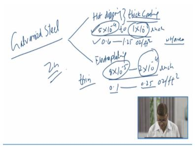
Galvanized steel: So basically there are 2 methods which are used for galvanizing. One is the hot dipping method. And another is electroplating in order to provide the coating of the zinc on to the surface of steel. Hot dipping method in general leads to the development of very thick coating. And if the larger amount of the zinc is getting into the weld it will be more problematic from the weldability point of view.
