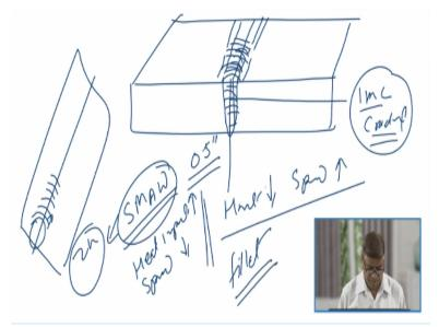
And to understand this we need to see the way by which two processes work like these are the sheets which are being applied. Since the SMAW process like this the plates being welded this is the line of the weld. So when the GMAW process is applied the heat input is less, the welding speed is more. So as a result of this whatever the zinc is present, most of the zinc will be going into the weld metal and promoting the IMC formation leading to the increased cracking tendency.
