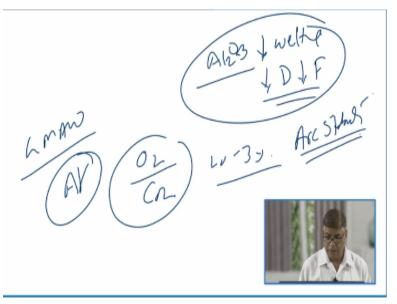
It may reduce the wetting of the molten metal. It may reduce the ductility and the formability of the weld joints. So effective protection of the weld metal from the atmospheric gases is needed in order to avoid the adverse effects.
