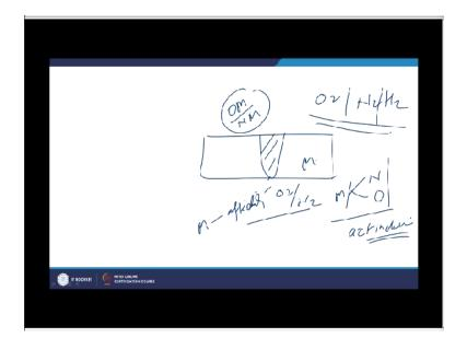
The chemical affinity is the another important aspect that I will explain little bit like if there is a metal system which is subjected to the external heat for the fusion. So, at high temperature there will be environmental gases like oxygen, nitrogen and hydrogen, so the way by which metal has the affinity to these gases which are present all around during the welding it can lead to the formation of the oxides of the metal or the nitrites of that given metal.
