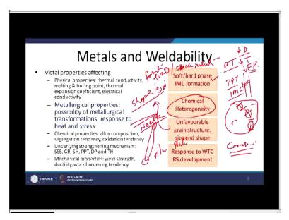
Sometimes what we see that during the metallurgical transformation some of the precipitates are formed or sometimes inter-metallic compounds are formed and formation of these precipitates and inter-metallic compounds either in the weld metal or in the heat affected zone will be leading to the localized enrichment or the deficiency of the alloying elements, like say this is one grain this is another.
