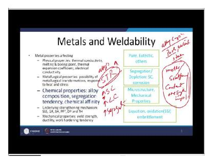
Now will see the next property of the material we know that if we say chemical composition which considers the alloy composition. So metal which is to be welded it is composition certainly plays a very big role in determining the weldability. It metal can be pure or it can be of the eutectic composition or other composition. So we that the pure metals and the eutectic alloys, alloys of the eutectic composition will be melting and solidifying at constant temperature at single temperature.
