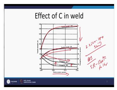
So, that is what this what we will see in this diagram this is the same diagram showing the variation in the tensile strength and ductility as a function of the carbon content for 2.25 chromium, 1 molybdenum steel. In as welded condition as well as in stress relived condition at 1300 Fahrenheit for 1 hour per section thickness. So, what it shows that is significant increase in the tensile strength in as welded condition.
