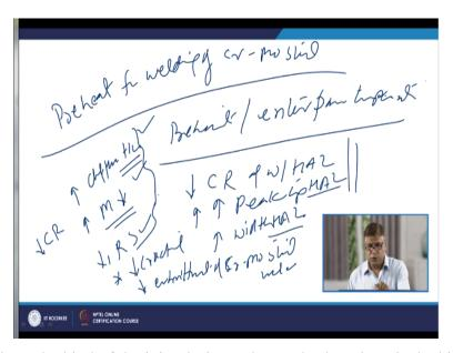
So, so that was about the kind of the joint design to be used. Then there is the kind of the preheat which is needed for welding of the chromium molybdenum steels. You know whenever we apply preheat, preheating of the plate or preheating of the base metal or then temperature. Whatever preheat is there the same is the inter pause temperature is used, whenever preheat is applied it will be lowering down the cooling rate of weld as well as the heat affected zone, this is one thing.
