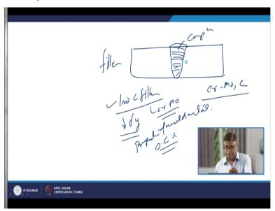
As for as the filler metal is concern the weld metal composition and accordingly the welding metrology to a great extent is influenced by the composition of the weld metal so, we know that since the chromium molybdenum and carbon content in the base metal is high, so we will prefer to use the low carbon fillers. But low carbon fillers will be leading to the reduction in the yield strength of the weldment and if this is acceptable from the service point of view.
