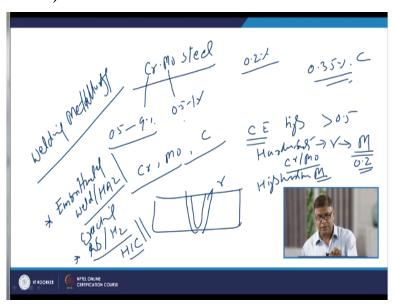
Now we will try to see the way by which the kind of the welding metrology involved in welding of the metrology involved in welding of the chromium molybdenum steels. We know that the chromium in these steels can range from 0.5 to 9% while molybdenum usually 0.5 to 1% while
