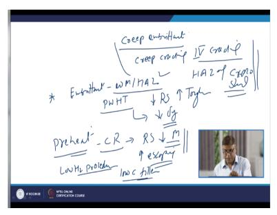
Hard and unique kind of the aspect which is observed related with this type of the welding is at the creep embrittlement. This is basically associated with the creep crack formation this is also known as a type 4 cracking and this is commonly observed in the heat affected zone of the chromium molybdenum steel weld joints. So, about this also we will be trying to will be talking that what are the factors that lead to the creep embrittlement.
