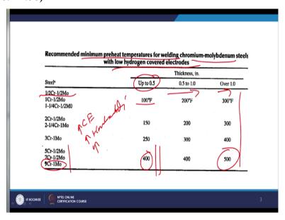
So this what we can see here this table shows the kind of preheat temperatures to be used when welding chromium molybdenum steels using the low hydrogen covered electrodes. So, say 0.5 chromium and 0.5 molybdenum is 100 Fahrenheit up to 0.5 inch thickness, 100 degree
