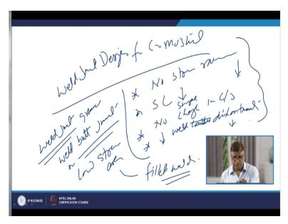
Therefore weld joint design for chromium molybdenum steel this must design must ensure that they are no stress razors, stress concentration is minimized. As well as well as there is no sharp change in cross-section at the toe of the weld or in the cross-section of the component or they are minimized the weld discontinuities are minimized.
