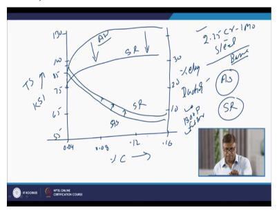
That is what we will try to see here from the simple diagram what it shows like carbon content is 0.04, 0.08 0.12 and say 0.16, this is weight percent of the carbon in increasing amount. In the y axis I will say this side we have the strength of the weldment increasing from say this is the minimum level 55KSI. So, the tensile strength KSI in case a unit say here it is 75 somewhere here 85 then 100 then 130 say this is 65.
