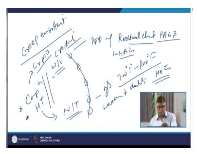
Now will be talking about the creep embrittlement basically is attributed basically it is attributed to the precipitation of residual elements at prior austenite grain boundaries in the heat affected zone. So, at the grain boundaries some of the undesirable phases precipitates and form the intermetallic compounds and the phases which at high temperature exposure on.
