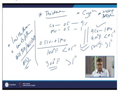
So, the kind of preheat to be used is directly found a function of the thickness and composition. So, these are the 2 main factors that affect the magnitude of the preheat thickness and the composition at the same time it the preheat temperature is also affected by the welding procedure. If we are using the low hydrogen procedures then the lower preheat temperature can be used.
