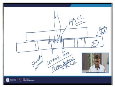
Now we will see the kind of when the plates are welded like this the groove which is being made then proper backing is given. So, for giving various space to provide the backing plate during the welding of the heat treatable low alloy steels. We may use the ceramic tape or we may use the copper backing with the holes from the bottom.
