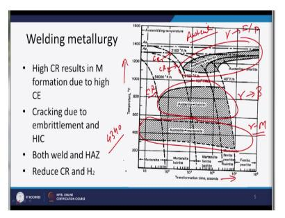
And what we can see when the steel is heated to the high temperature and leading to the formation of the austenite. What happens to the steel when it is cooled at the different rates, what we can see there are 3 zones in this continuous cooling diagram. One zone is this one where the different phases are being formed the cooling rate is low and this zone corresponds to the transformation of the austenite into the ferrite as well as pearlite.
