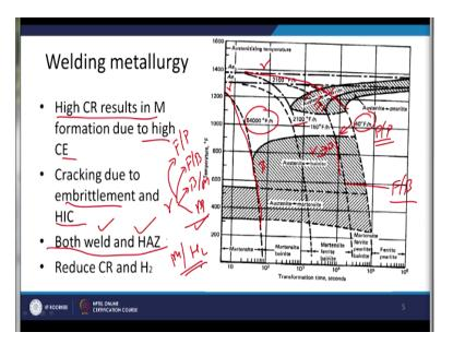
So, if we try to understand what happens when the steel is cooled very slowly say that is this case, when the steel is being cooled very slowly leading to the. So, first the austenite transforms into the ferrite in this bend of the time zone and then the remaining austenite transforms into the pearlite. So, in this case primarily will be having the ferrite and the pearlite in the micro structure of steel when it is cooled at like say 40 degree Fahrenheit/hour.
