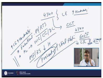
And as a result of this leading to the higher carbon equivalent leading to the higher hardenability. So, now in order to understand the relationship between the kind of micro structures which are observed during the welding in heat treatable low alloy steels and there the possible performance or it is effect on the weldability. And that we can understand in much better way using the continuous cooling diagram or CCT diagram.
