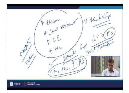
So, in general when we work with the greater thickness of the plate and when the joint restrained, joint restrained conditions when the joint is being made is high. And the carbon equivalent is high, section thickness is high and when the hydrogen content in the weld is high all these will be increasing the preheat temperature requirement. And when it is possible to apply the suitable preheat then preheat temperature selected must be about 50 degree Fahrenheit greater than the Ms temperature.
