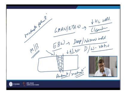
On the other hand like if we are using the processes like GMAW and the GTAW processes both these processes offer low hydrogen weld joints. So, in general the weld is cleaner and we are able to produce the weld joints which will be less prone to have the defects and discontinuities. When the electron beam welding process is used for welding of the heat treatable low alloy steels it is possible to have the very deep penetration and very narrow weld.
