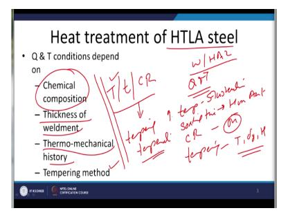
Now we will see the kind of the heat treatment which is given to the Q and T steels, so that the properties can be restored that will depend upon the number of these parameters.
