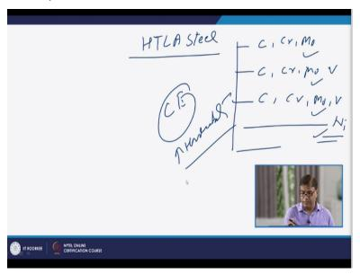
Now we will see the heat treatable low alloy steels significantly differ in terms of the kind of the elements which are present in 8, they are various categories of the Q and T steels few will be having higher carbon, chromium, molybdenum only. While others will have carbon, chromium, molybdenum and vanadium also while there is category of the heat treatable low alloy steels which will have carbon, chromium, molybdenum, vanadium as well as nickel.
