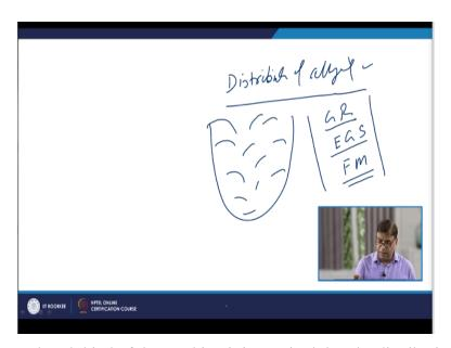
So, in order to control such kind of the cracking it is required that the distribution of the alloying elements is maintained properly and the segregation is avoided. And for that if the molten metal flow in the weld metal is maintained in such a way that the such kind of the segregation tendency is reduced then that will help in controlling the solidification cracking tendency.
