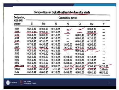
So, if we see here 4130 and then 4340 these are the few categories of the steels which are extensively commonly used. So, if we take a 4340 steel having the carbon 0.38 to 0.43 manganese 0.6 to 0.8 this is having the nickel of 1.6 to 2%, chromium is 0.7 to 0.9, molybdenum is 0.2 to 0.3. This is one type of the steel there is like 4037 steel having the carbon 0.35 to 0.4, manganese 0.7 to 0.9, there is no nickel, there is no chromium, molybdenum 0.2 to 0.3.
