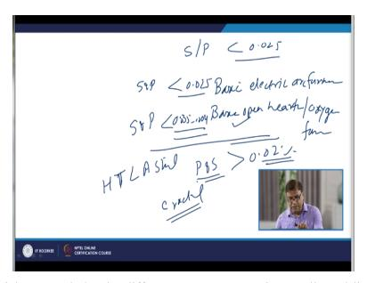
So, the steels which are made by the different processes, maximum allowed limit normally this should be less than 0.025% but for both sulfur and phosphorus. But the steels prepared using the process like the basic electric arc furnace. The maximum the sulfur and phosphorus content should be less than 0.025. While in case of the basic open hearth and oxygen furnaces the maximum allowed limit is less than 0.035 to 0.04.
