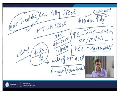
And reason for this is that the heat treatable low alloy steels, in short this is written as HTLA steel. This is these steels have the much higher hardness then the other category of the steels much higher yield strength. And these properties come basically from the higher percentage of the carbon content in these steels which ranges from the 0.25 to 0.45% along with the greater percentage of the chromium molybdenum and nickel.
