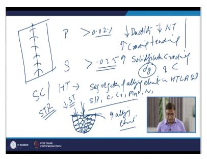
So, the phosphorus whenever it is present in quantity greater than 0.02% in steel it decreases the ductility of steel it decreases the notch toughness of the steel. And because of this the cracking reduced ductility and toughness promotes the cracking tendency of the steel. On the other hand when the sulfur is greater than 0.025% or 0.02% it increases the solidification cracking tendency of the weld metal.
