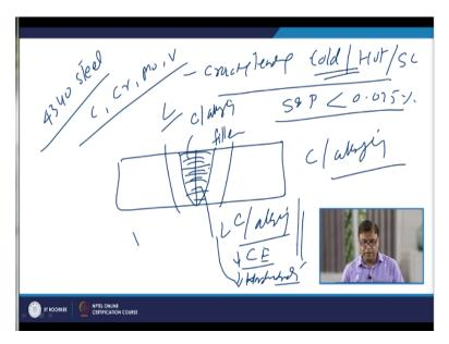
Now we will see there is one typical category of the heat treatable low alloy steel that is 4340 steel. This steel has the higher carbon, higher chromium, molybdenum, vanadium percentage and because of the higher concentration of these alloying elements it shows the cracking tendency. Both cold cracking as well as hot cracking or the solidification cracking tendency.
