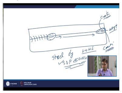
Now we will see that during the welding when the welding is performed so the weld metal is deposited like this and the molten metal pool will be moving in this manner. So, when this portion when the pool reaches means as soon as the welding is completed and we reach at the end of the weld center lines. So, near the end where the weld terminates this zone is the crater where we will see the alloying concentration is high.
