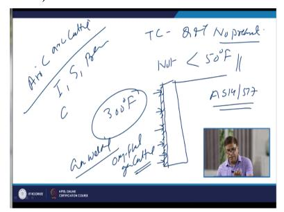
Normally, so as I said normally in case of the thermal cutting of these Q and T steels no preheat is needed, provided the plate temperature is not less than 50 degree Fahrenheit. If the plate temperature is less than 50 degree Fahrenheit then we must preheat at least this temperature. But in some cases like the steels of the high yield strength like A514 or A517 steels which are of the high yield strength, higher concentration of the alloying element.
