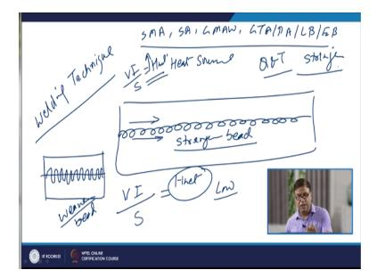
So, as for as the welding technique is concern like there can be number of processes which can be used for depositing the weld metal submerged arc welding shielded metal arc welding. Then gas metal arc welding and non consumable processes like GTAW and the PAW processes then laser beam and the electron beam welding processes. But metal is being applied and how the heat source is being applied during the welding.
