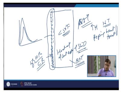
So, whatever the method of the cutting is being used, it the thermal cutting using the air carbon arc cutting method or air plasma cutting method. Basically the kind of the thermal cycle experienced by the cut edge will be similar to that of the welding except that here only one side of the edge is being affected due to the thermal cycle. So, thermal cycle for which the base metal being exposed is similar to that of the welding.
