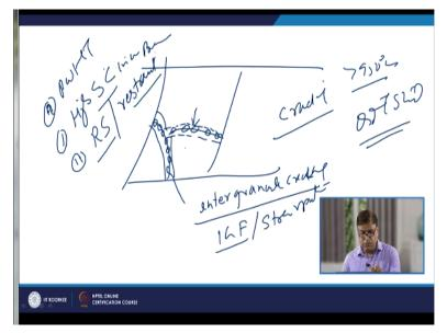
So basically since these this kind of the precipitation takes place at the grain boundary like say this is the heat affected zone. And here precipitation has taken place at the grain boundary and these boundaries. So, the grain boundary area is weakened, so the cracks start to propagate along the grain boundary because of precipitation of these unfavorable carbides especially at the grain boundaries.
