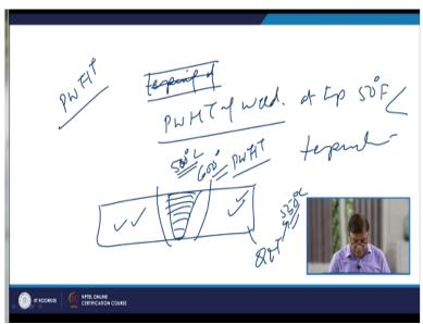
In any case if the PWHT is to be carried out of the entire assembly in order to restore the complete set of the properties. In that case the tempering of the or you can say not tempering but PWHT heat treatment of the weld joint is carried out at temperature about 50 degree Fahrenheit less than the tempering temperature, why. Because like say this is the weld joint this is the plate and this is the weld joint which has been made.
