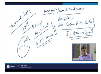
Now we will talk about the another aspect related with the thermal processing of the Q and T steel is thermal cutting. Like frequently it is required to cut the required size of the blank from the large size plate, so that these can be further processed in order to get the desired size and shape of the component. So, we can use the mechanized or manual thermal cutting.
