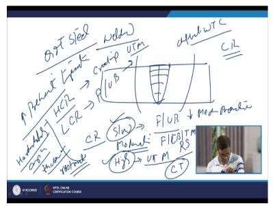
Now we have seen that when the Q and T steels are welded or when welding is performed you know the weld metal as well as the heat affected zone say this is weld metal and the heat affected zone . These will be experiencing the different weld thermal cycles in the different zones and the kind of cooling rate which is experienced in these cases.
