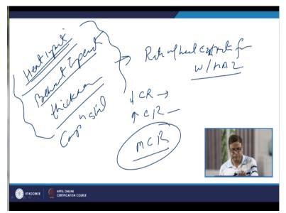
Now we will see the heat input related aspect, heat input and the preheat temperature and the thickness of the plate. These are the 3 aspects which are seen together because a combination of these 3 will be determining the rate at which rate of heat extraction from the weld as well as heat
