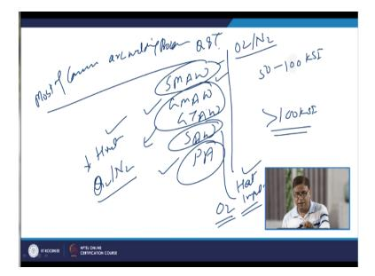
Now we will be talking about the processes which are available like most of common arc welding processes can be used for welding of the Q and T steels like SMAW, GMAW, GTAW, SAW, PAW all these can be used for welding of all types of steels having the strengths from 50 to 100KSI. But when this is the very general statement but when the steel strength is greater than 100KSI we would like to use those good quality welding processes which offers the lesser heat input.
