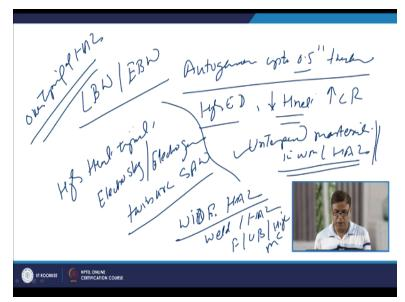
We can use the laser beam welding and electron beam welding for autogenous means direct welding, no filler autogenous welding up to 0.5 inch thickness of the Q and T steels. Since the both these processes are of the very high energy density, so they will supply very less heat for realizing the fusion of the faying surfaces to develop the joint, cooling rate is extremely high.
