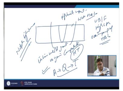
So, in order to overcome the issues related with the weld joints made using the high heat input processes like wide Hz upper bainide, ferrite and high carbon martensite or even over tempering of the Hz. It is required that entire weld joint is given complete heat treatment again what it involves austenitizing of the weldment followed by quenching then tempering.
