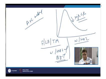
Otherwise in most of the arc welding processes the kind of weld thermal cycle which is realized in the weld as well as heat affected zone it is such that cooling rate is high enough to form the ferrite, lower bainide and the tempered martensite auto tempered martensite in the weld as well as heat affected zone of the Q and T steel weldments. And that is why the mechanical properties of the weld and as well as Hz of the Q and T steels are similar to that of the base metal.
