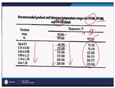
And in the next slide we have few more the preheat and interpass temperatures for HY80, HY100 and HY 130 steels. And what we notice that in this case also with increase in thickness of the plate required preheat temperature is also increased. So, almost similar kind of the preheat temperatures are there for HY80 and HY100 like up to 0.5 inch it is 60 to 300 Fahrenheit then 125 to 300.
