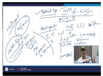
So, **so** we have to fix up at least one thing like preheat temperature is fixed say 100 Fahrenheit for a 25mm thick plate. Then for this preheat inverse for this thickness of the plate of a given steels say A514 B grade steel. Then we need to establish the heat input for the process which is being selected and heat input how can we choose now for all those arc welding processes heat input is obtained through the voltage into current gives us the power of arc or in the joule.
