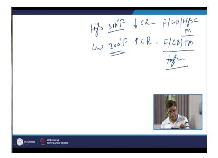
And therefore the different value of the preheat is used say too high preheat temperature say 500 Fahrenheit will be lowering down the cooling rate which will be leading to the formation of the ferrite upper bainide and maybe a high carbon martensite. On the other hand low cooling rate will be leading to the like say 200 Fahrenheit, so this 200 Fahrenheit will be leading to the reasonable cooling rate and good combination of the ferrite lower bainide and the maybe tempered martensite.
